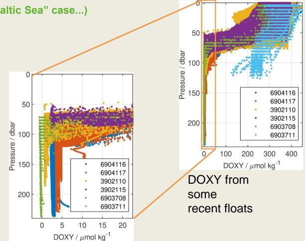
Zoom on low DOXY range: Should be zero  $O_2$  in  $H_2$ S-containing deep waters -> OFFSET correction needed
