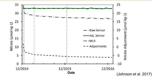
**Figure 5.** Nitrate sensor data at 1500 m depth for float 5904469/9096 and the predicted (MLR) nitrate concentrations. Dashed line shows the adjustments that are applied to the raw sensor data. Vertical dotted lines are locations of four nodes where changes in the adjustment parameters in Table 5 are applied.
