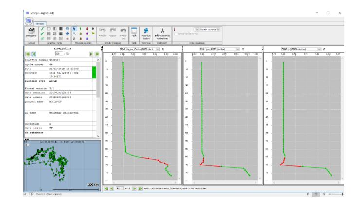
**Digit rollover test:** The digit rollover test is a remnant from early Argo days when only a limited amount of bits were available for transmission in the Argos satellite system. The range of encountered temperature and salinity data however was not always large enough to accommodate them and when the range was exceeded stored values rolled over to the lower end of the range.
