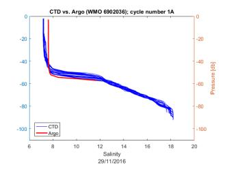
**Step 5:** Run **IOPANmeanDMQC.m** script that calculates, for each Argo profile and the closest CTD profiles, the mean salinity in the selected layer (S=10-30 m, T=70-90m) and difference between them.
