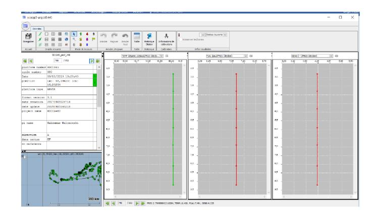
Gradient test: This test had been designed to assign a 'bad data' quality flag when the difference between vertically adjacent measurements is too steep and has the potential to catch strong gradients in deep layers of the Baltic caused by the inflowing North Sea waters. It was declared obsolete in October 2019 at ADMT20 but it seems that the data from the Baltic floats need to be reprocessed to accommodate this decision.
