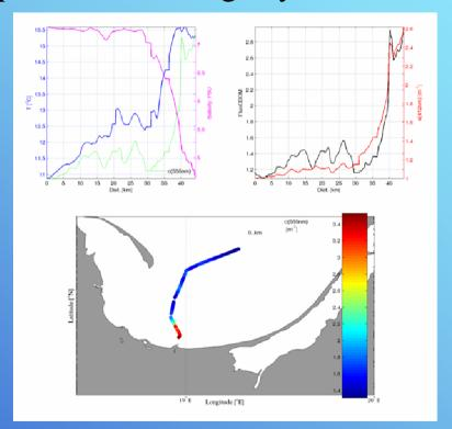
Examples of the horizontal distribution of salinity temperature, spectral absorption and attenuation coefficients and CDOM fluorescence in the Gulf of Gdansk (not calibrated, in DC fluorometer output).
