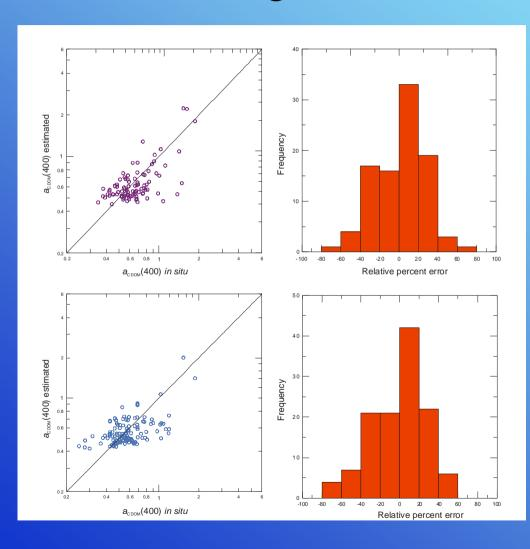
Upper panel: validation results of the Kowalczuk et al. (2005) algorithm using spectral reflectances derived from SeaWiFS ocean color imagery: Bias = 0.02, RMS = 0.23,  $R^2 = 0.50$ , n = 97. The lower panel validation results of the Kowalczuk et al. (2005) algorithm using spectral reflectances derived from MODIS ocean color imagery: Bias = 0.03, RMS = 0.19,  $R^2 = 0.38$ , n = 122.
