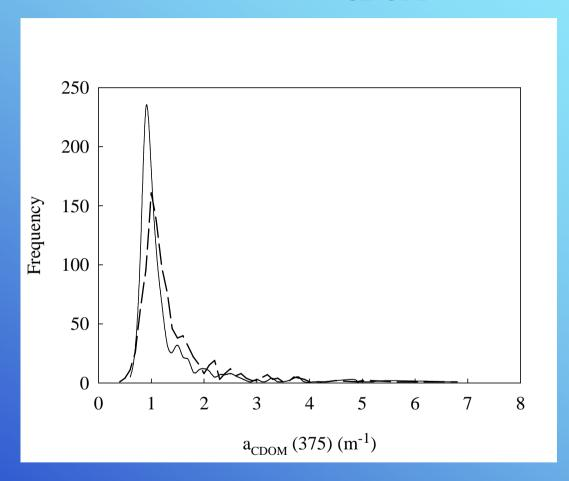
Distribution of  $a_{\rm CDOM}(375)$  values calculated using two different baseline correction approaches; inclusion of constant "K" in a non-linear regression procedure (solid line) and subtraction of average absorption value between 650-700nm (dashed line).
