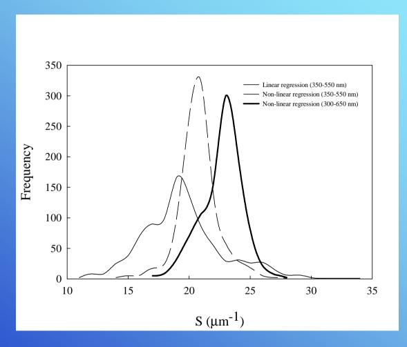
Distribution of S estimates from the three different approaches applied: linear regression in the spectral range 350-550 nm (thin solid line), non-linear regression, spectral range 350 - 550 nm (dashed line), non-linear regression in spectral range 300 - 650 nm (thick solid line).
