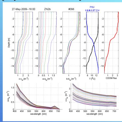
Examples of the vertical profile of salinity temperature, spectral absorption and attenuation coefficients and CDOM fluorescence (not calibrated, in DC fluorometer output)
