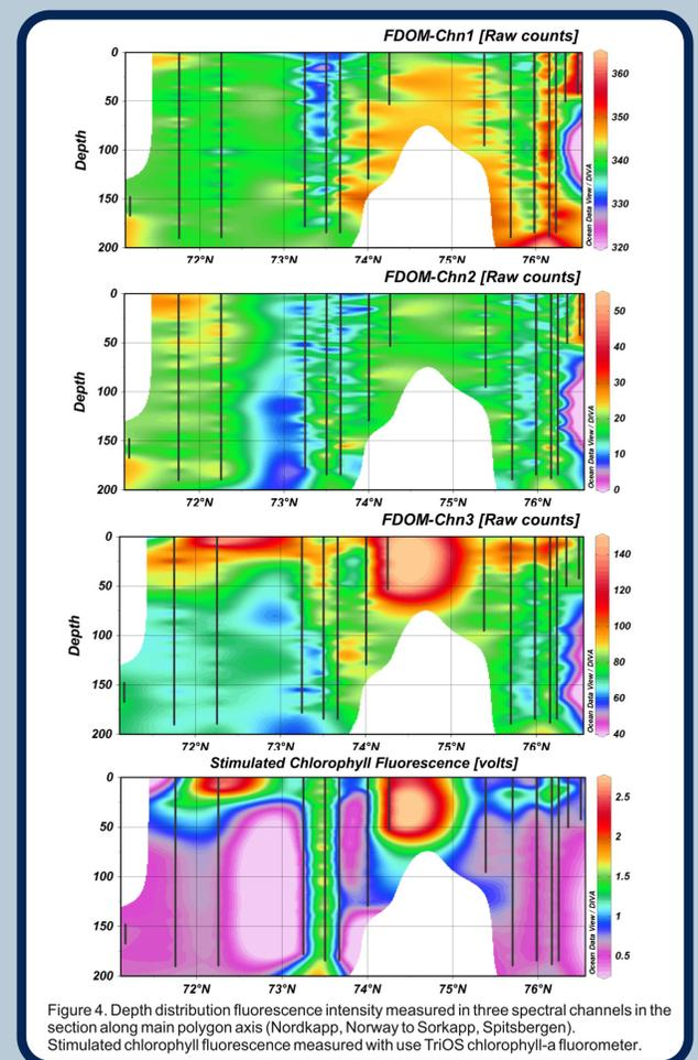
Figure 4. Depth distribution fluorescence intensity measured in three spectral channels in the section along main polygon axis (Nordkapp, Norway to Sorkapp, Spitsbergen). Stimulated chlorophyll fluorescence measured with use TriOS chlorophyll-a fluorometer.
