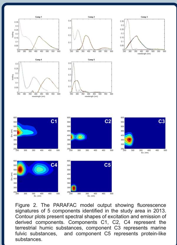
Figure 2. The PARAFAC model output showing fluorescence signatures of 5 components identified in the study area in 2013. Contour plots present spectral shapes of excitation and emission of derived components. Components C1, C2, C4 represent the terrestrial humic substances, component C3 represents marine fulvic substances, and component C5 represents protein-like substances.
