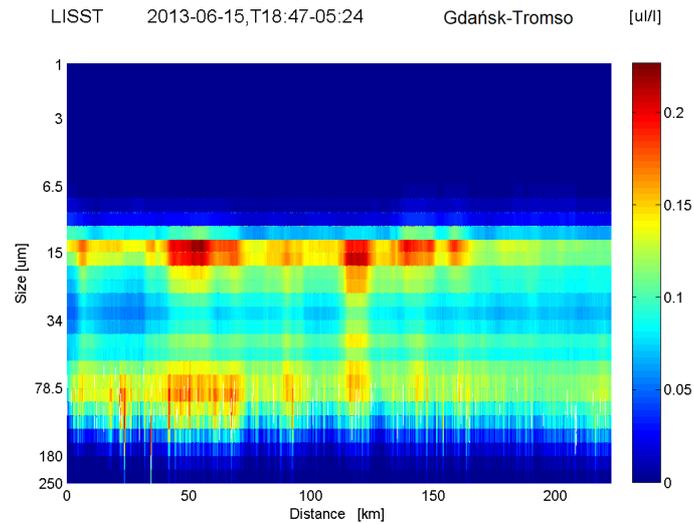
Fig. 4 Example spatial distribution of volume particle concentrations (measurement 4 and 6) of the Arex2013/1 cruise. Size distribution for 32 size classes in range of 1.2 to 250 µm, logarithmic scale.
