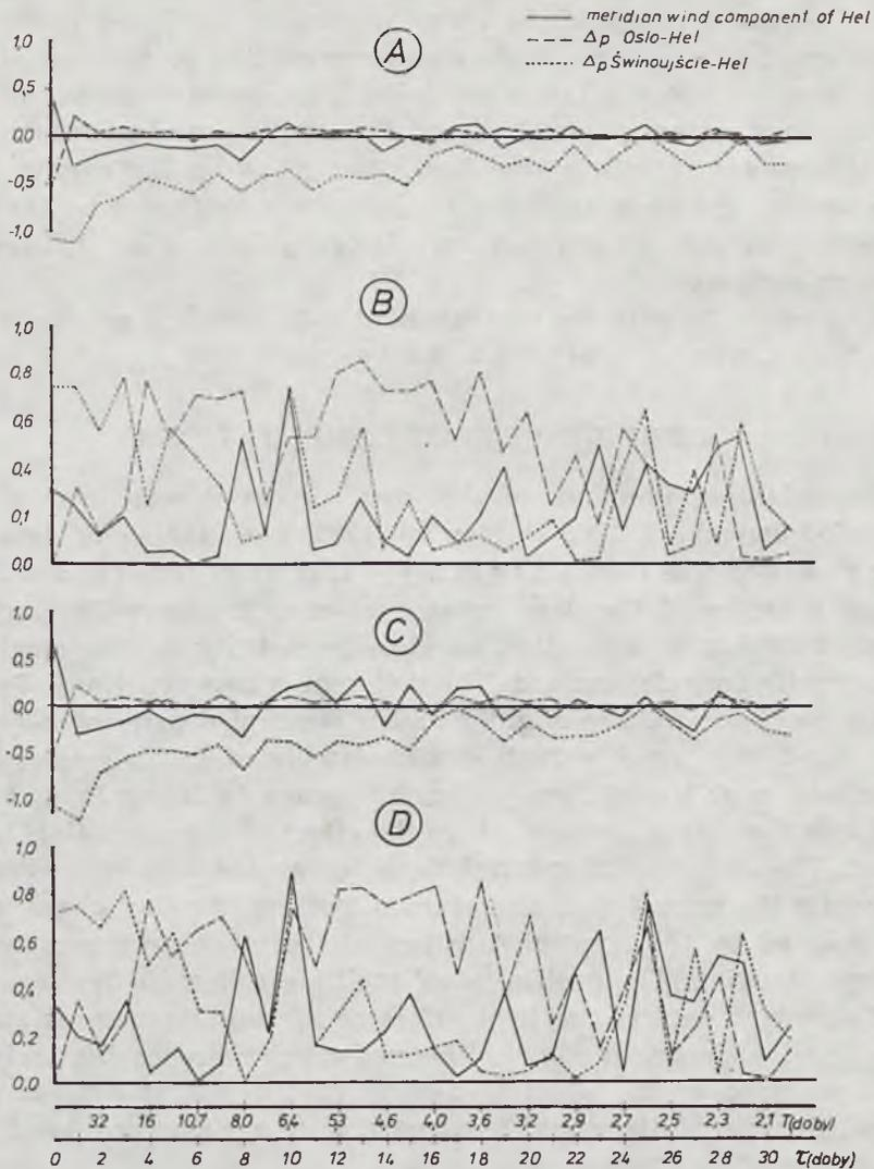
Fig. 4. Weighting functions (A) and partial coherences of input processes (B) for Hel, also weighting functions (C) and partial coherences of input processes (D) for Nowy Port
