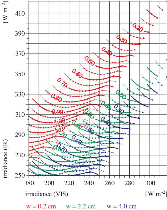
**Fig. 4.** The dependence of the zenithal aerosol thickness  $\tau_{aer,1+2}(550)$  (isolines) found by the pyranometric method on the input parameters: the VIS and IR irradiance, and the precipitable water vapour in the zenithal path  $w$ . Computations for  $\vartheta = 45^\circ$
