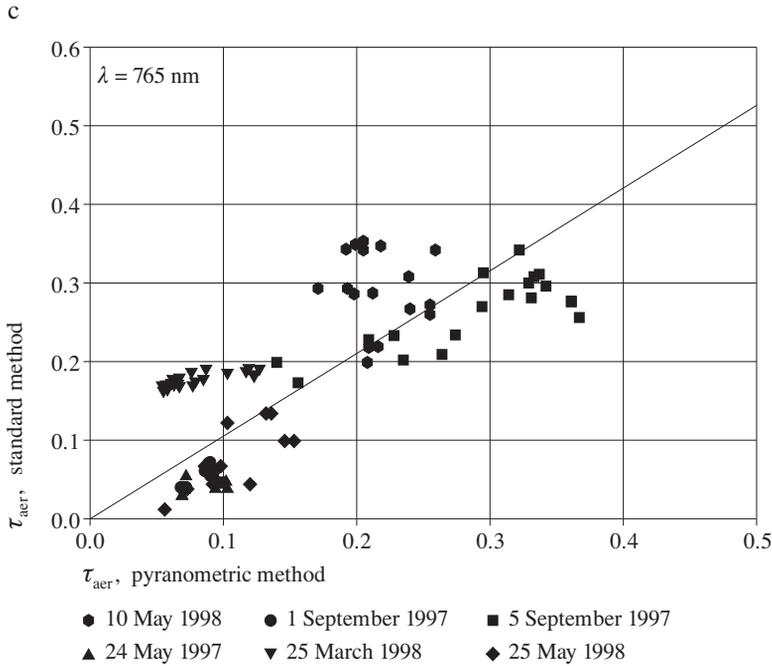
**Fig. 2.** Comparison of the zenithal aerosol optical thicknesses at  $\lambda = 443 \text{ nm}$  (a),  $\lambda = 555 \text{ nm}$  (b),  $\lambda = 765 \text{ nm}$  (c), obtained by the standard and pyranometric methods. Measurement points from one day are denoted by the same symbol
