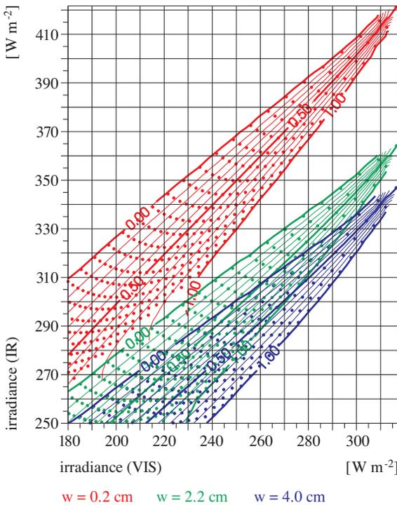
**Fig. 5.** The dependence of the parameter  $\frac{\tau_{aer,1}}{\tau_{aer,1}+\tau_{aer,2}}$  (isolines) found by the pyranometric method on the input parameters: the *VIS* and *IR* irradiance, and the precipitable water vapour in the zenithal path  $w$ . Computations for  $\vartheta = 45^\circ$
