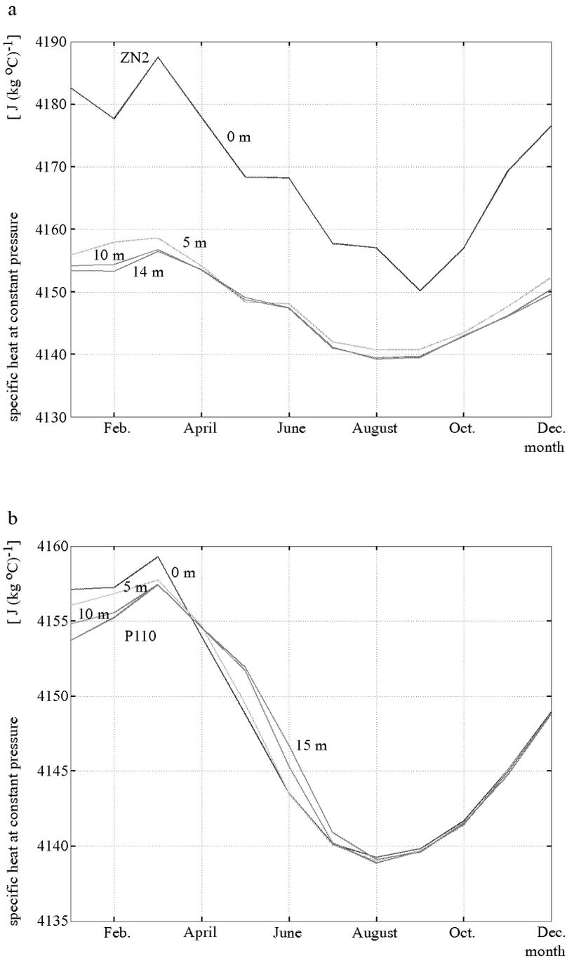
Fig. 4. Annual variation in specific heat at constant pressure of seawater at stations ZN2 and P110 at depths of 0, 5, 10 and 14 (15) m
