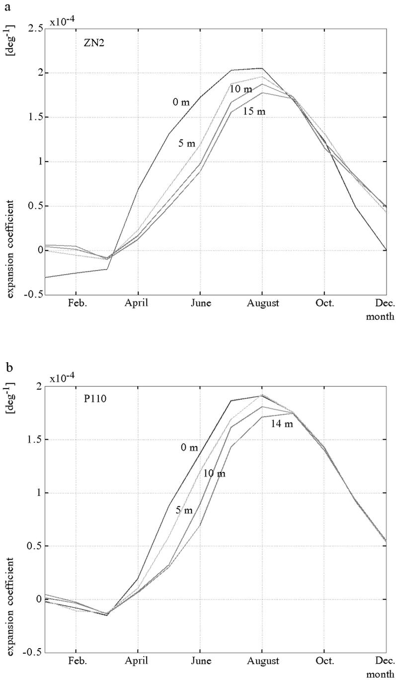
Fig. 5. Annual variation in the seawater expansion coefficient at stations ZN2 and P110 at depths of 0, 5, 10 and 14 (15) m
