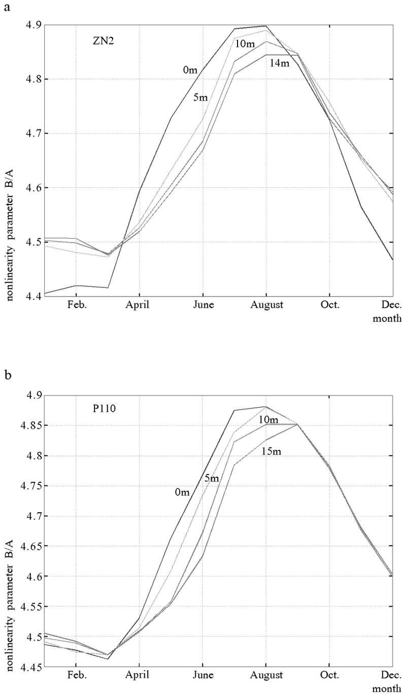
Fig. 8. Annual variation in the nonlinearity parameter  $B/A$  at stations ZN2 and P110 at depths of 0, 5, 10 and 14 (15) m
