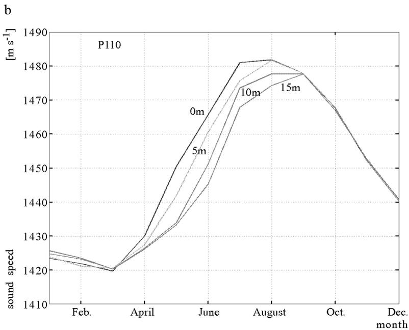
Fig. 7. Annual variation in the speed of sound at stations ZN2 and P110 at depths of 0, 5, 10 and 14 (15) m
