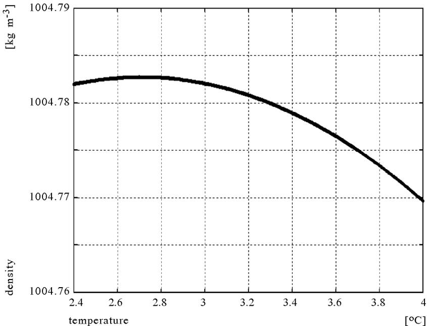
Fig. 14. Density of water of salinity 6 psu as a function of temperature
