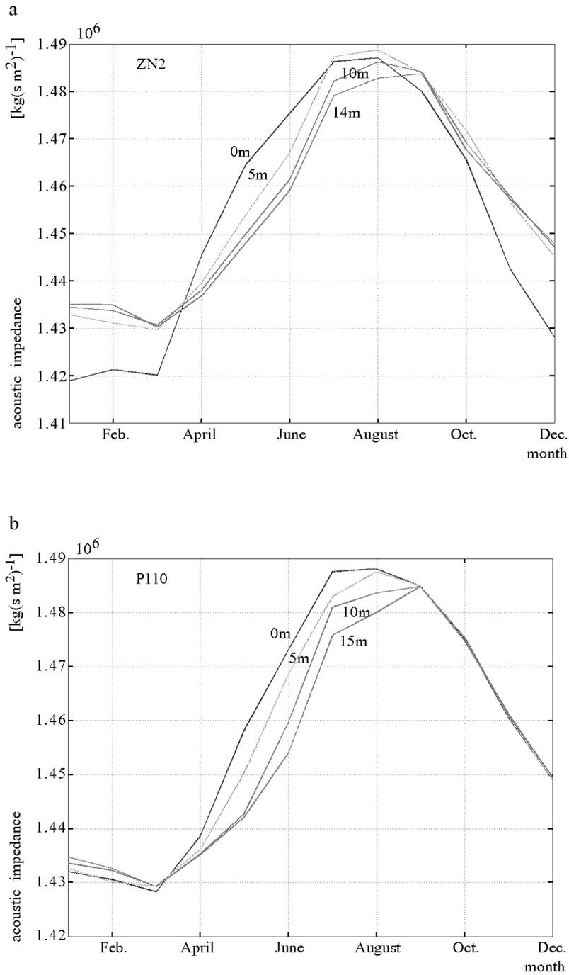
Fig. 9. Annual variation in acoustic impedance at stations ZN2 and P110 at depths of 0, 5, 10 and 14 (15) m
