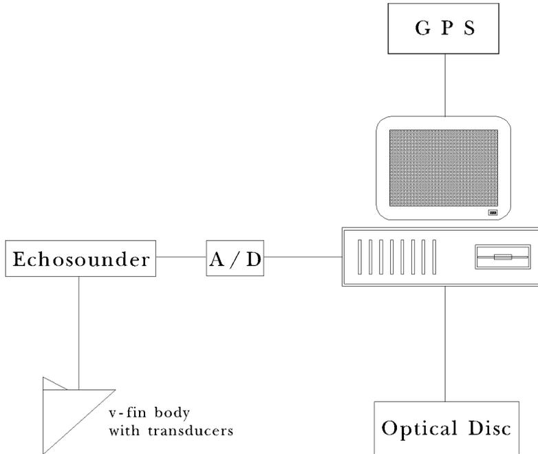
Fig. 2. Block diagram of the measurement setup
