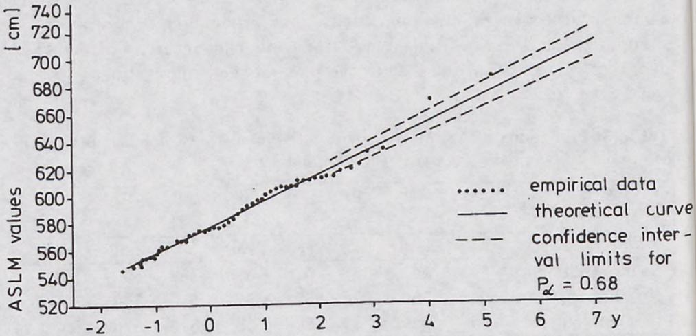
Fig. 6. ASLM probability distribution at Świnoujście (trend removed) computed by Gumbel's method
