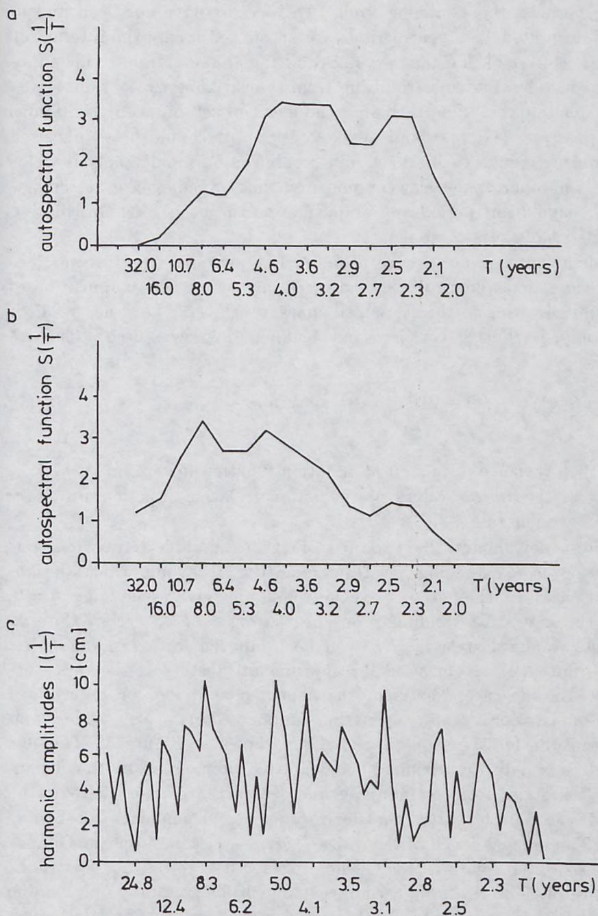
Fig. 4. Computations of ASLM periodic structure at Kołobrzeg. Computation of autospectral function (a), computation of autospectral function for the first differences (b), harmonic analysis (c)
