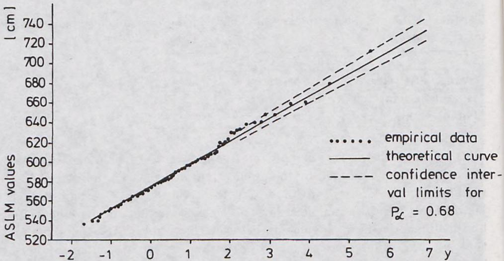
Fig. 7. ASLM probability distribution at Kołobrzeg (trend removed) computed by Gumbel's method
