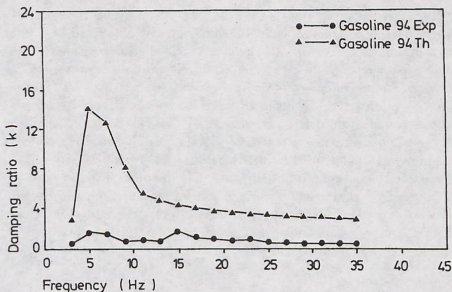
Fig. 1. The damping ratios of sea surface relationships versus frequency (1–40 Hz) in the presence of a Gasoline 94 film. The theoretical damping ratios are computed from equation (1) in which the static and dynamic parameters were taken from experimental measurements (reproduced by permission of Dynamics of Atmosphere Oceans)
