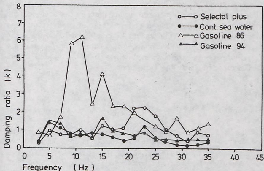
Fig. 3. Acoustically obtained damping ratios for the oil films studied versus frequency (1–40 Hz) under natural conditions and at wind speeds of  $u = 2\text{--}2.3 \text{ m} \cdot \text{s}^{-1}$  (reproduced by permission of Dynamics of Atmosphere Oceans)
