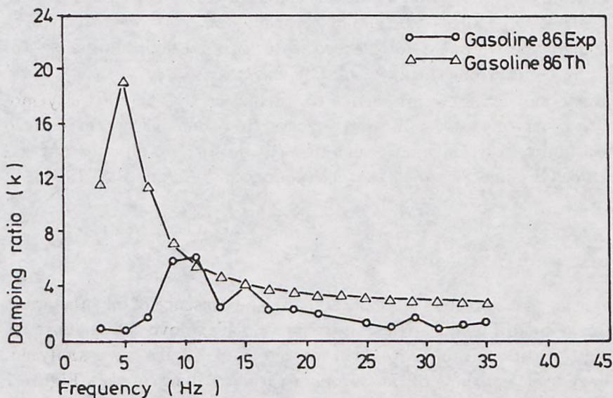
Fig. 2. The damping ratios of sea surface relationships versus frequency (1–40 Hz) in the presence of a Gasoline 86 film. The theoretical damping ratios are computed from equation (1) in which the static and dynamic parameters were taken from experimental data (reproduced by permission of Proceedings of the Conference Acoustical Imaging, Bohum, 1991)
