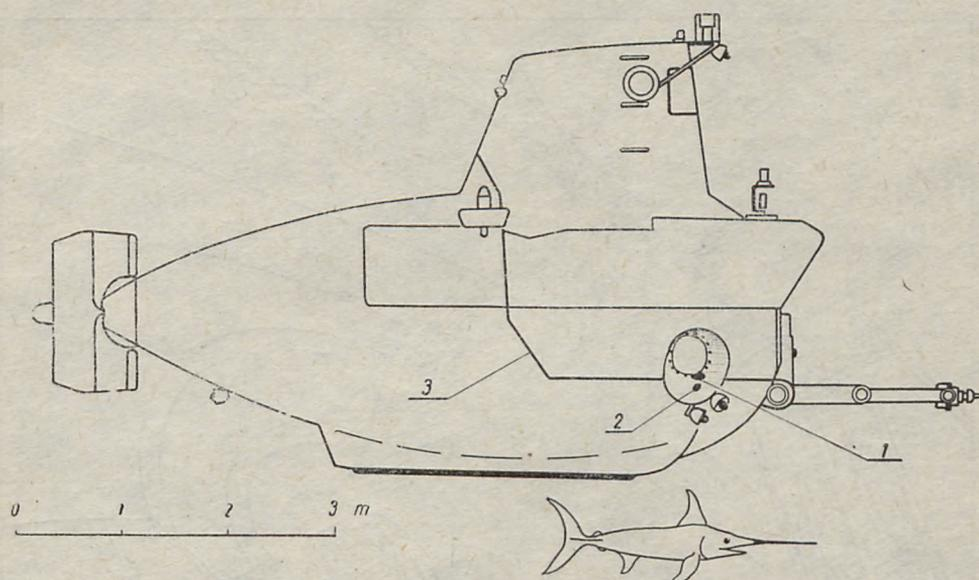
Fig. 2. ALVIN and the sword-fish drawn to scale, showing the location of the joint in the external, flooded hull of the submarine, the point of impact and the sword entry at the starboard window: 1 — sword wedged here, 2 — point of impact, 3 — junction in external (flooded) hull
