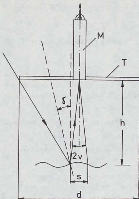
Figure 1: An outline of the geometry of upward radiance measurement above the sea surface:  $M$  - radiance meter,  $T$  - black screen,  $h$  - distance between the screen and the water surface,  $s$  - diameter of the observed fragment of the water surface,  $v$  - sight angle of the meter,  $\gamma$  - slope of the wave
