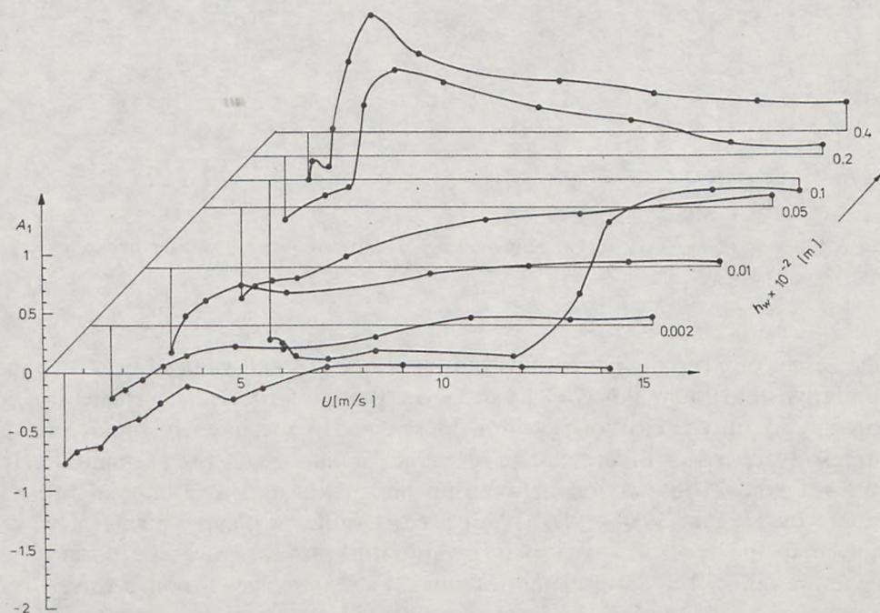
Fig. 7. Coefficient of asymmetry  $A_1$  of statistical distribution of amplitudes of signal scattered on a rough water surface covered with a layer of diesel oil vs  $h_w$  and  $U$
