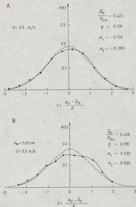
**Fig. 4.** Probability distributions  $P(t)$  of amplitudes of the acoustic signal scattered on a rough surface
