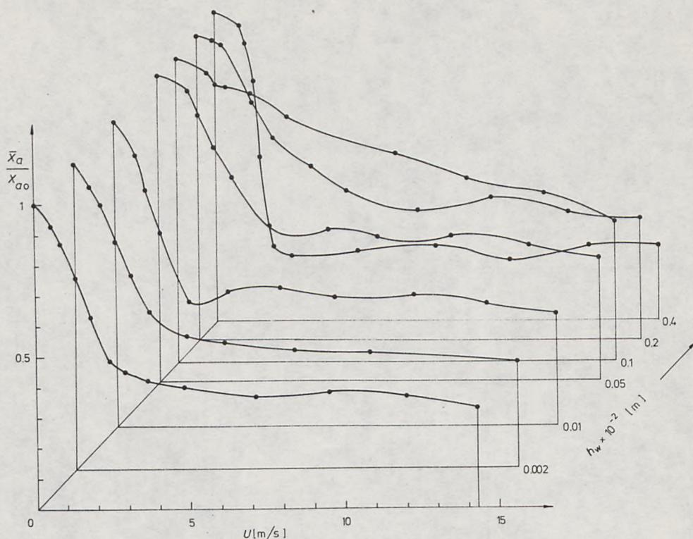
Fig. 5. Mean normalized amplitude  $\bar{X}_a/X_{a0}$  of signal scattered on a rough water surface covered with a layer of diesel oil vs  $h_w$  and  $U$
