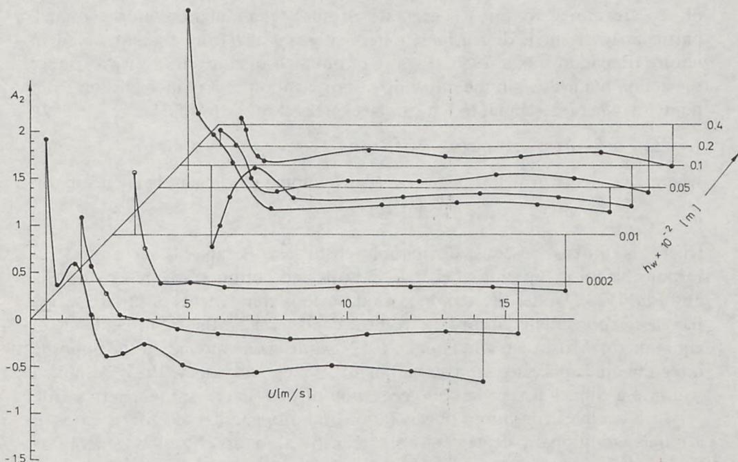
Fig. 8. Coefficient of flattening  $A_2$  of statistical distribution of amplitudes of signal scattered on a rough water surface covered with a layer of diesel oil vs  $h_w$  and  $U$
