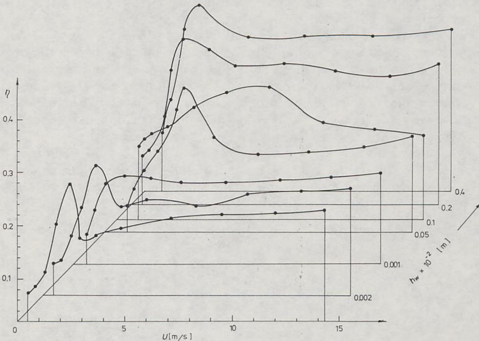
Fig. 6. Fluctuation coefficient  $\eta$  of amplitude of signal scattered on a rough water surface covered with a layer of diesel oil vs  $h_w$  and  $U$
