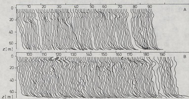
**Fig. 11.** Momentary vertical profiles of salinity measured at anchor station AN-2
