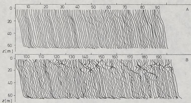
**Fig. 10.** Momentary vertical profiles of salinity measured at anchor station AN-1
