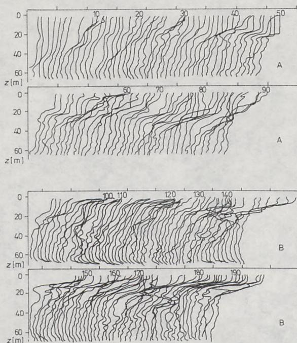
**Fig. 8.** Momentary vertical profiles of temperature measured at anchor station AN-1
