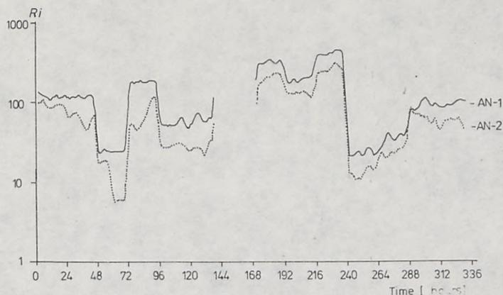
Fig. 13. Changeability of Richardson's number.  $\Delta z = z_2 - z_1 = 40 \text{ m} - 10 \text{ m} = 30 \text{ m}$
