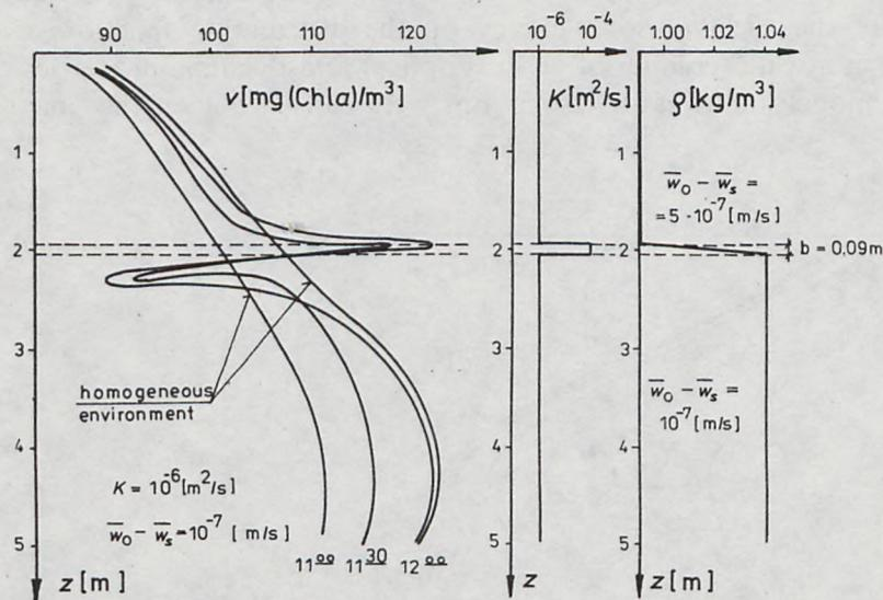
Fig. 7. Evolution in time ( $t$ ) of vertical distribution of chlorophyll  $a$  concentration under the conditions of suspension settling, existence of a fine stratification in density field and presence of a turbulent layer in a stable fine structure of thickness  $\delta = 9$  cm
