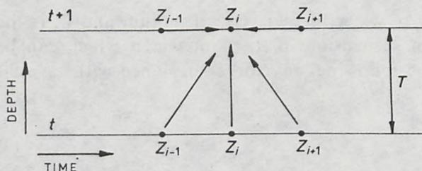
Fig. 4. Schematic diagram of a calculation net for the indirect Crank-Nicholson's method
