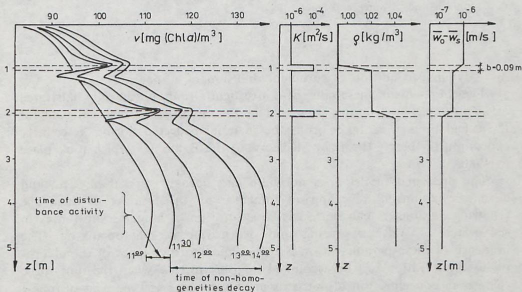
Fig. 9. The process of decay in time ( $t$ ) of structural non-uniformities in vertical distribution of chlorophyll  $a$  concentration under conditions of suspension settling
