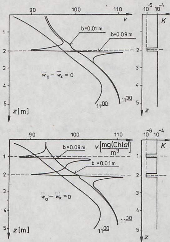
Fig. 11. The effect of the thickness of laminar interlayers on the intensity of formation of non-uniformities in vertical distribution of chlorophyll *a* concentration under conditions of suspension settling
