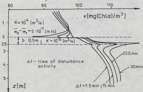
Fig. 12. Evolution in time ( $t$ ) of vertical distribution of chlorophyll *a* concentration under conditions of suspension settling and existence of a laminar interlayer of thickness  $\delta = 50$  cm in a turbulent velocity field
