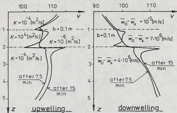
Fig. 13. Vertical distributions of chlorophyll *a* concentration in two instants of action of laminar interlayers of thickness  $\delta = 10$  cm in a turbulent velocity field and anisotropic suspension transport
