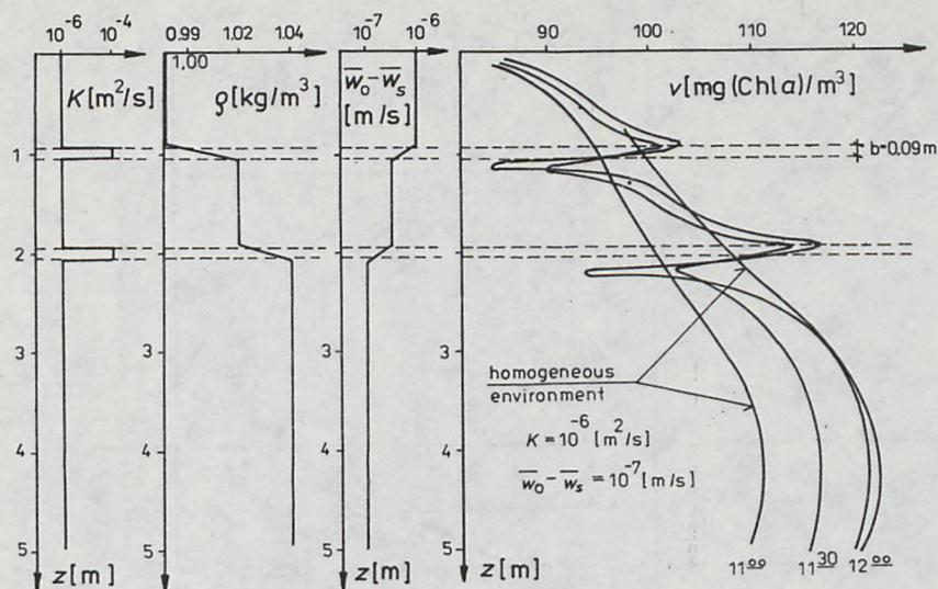
Fig. 8. Evolution in time ( $t$ ) of vertical distribution of chlorophyll  $a$  concentration under the conditions of suspension settling, existence of a fine stratification in density field and presence of two turbulent layers in stable structures of thickness  $\delta = 9$  cm
