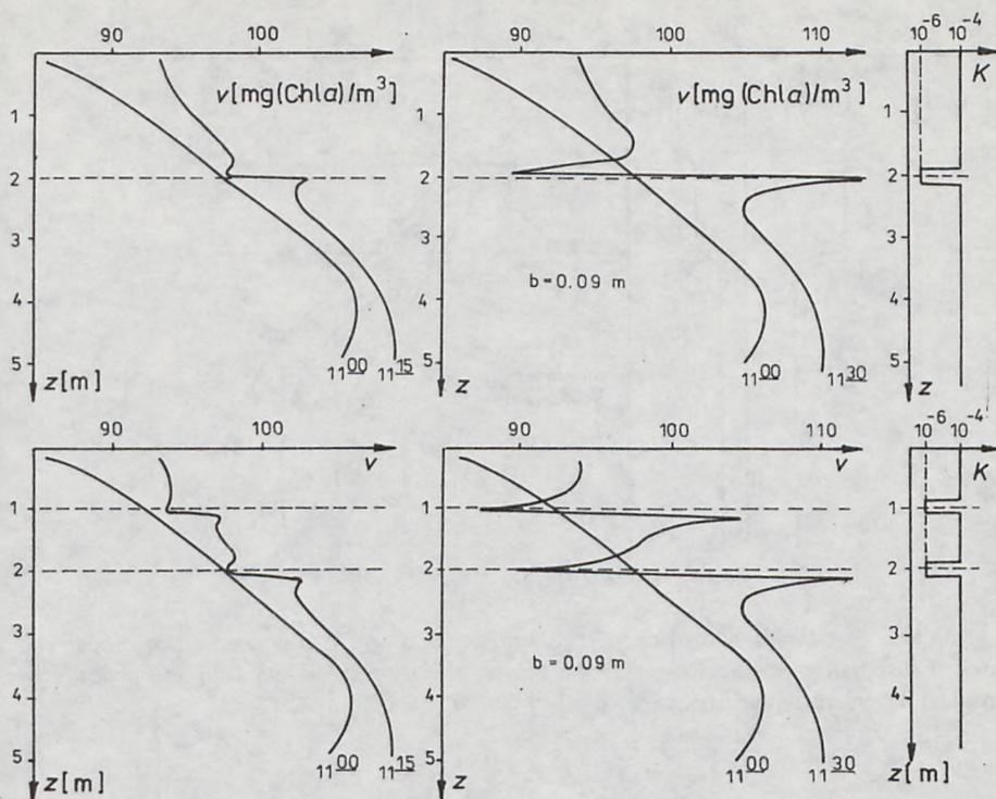
Fig. 10. Evolution in time ( $t$ ) of vertical distribution of chlorophyll  $a$  concentration under conditions of suspension settling and existence of fine laminar interlayers of thickness  $\delta = 9$  cm in a turbulent field of water horizontal flow
