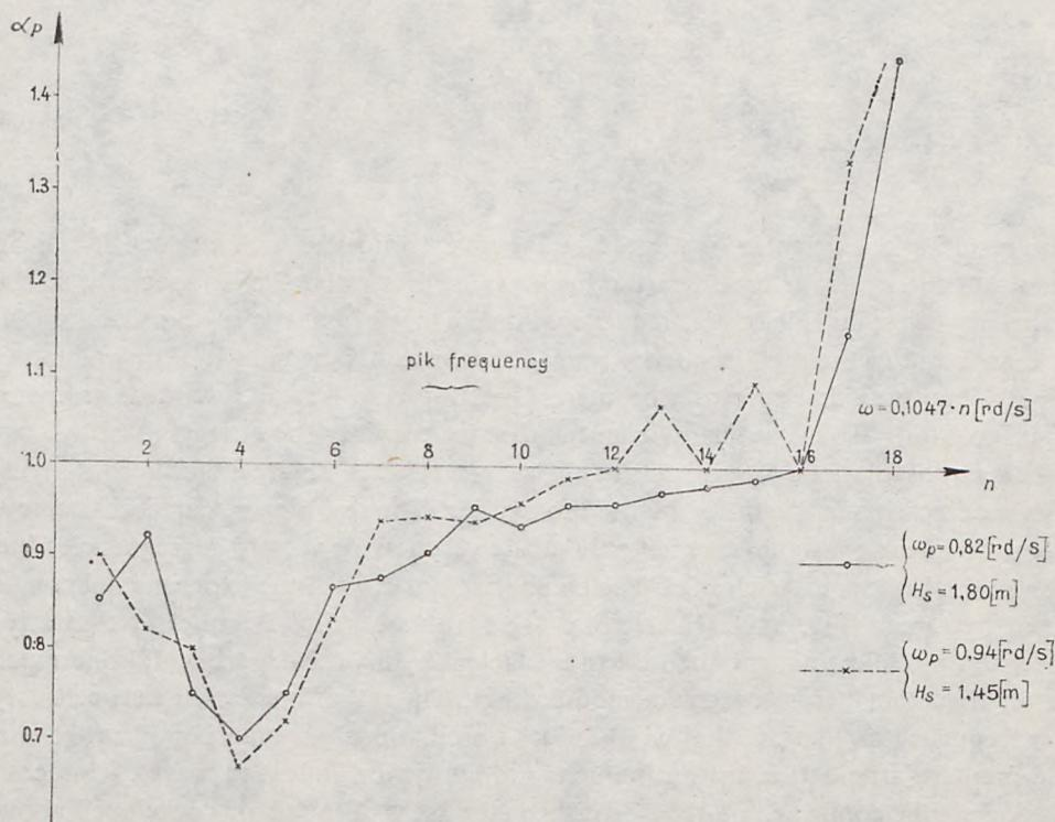
Fig. 5. Empirical coefficient  $\alpha_p$  for pore pressure in sandy sea bed, [20]
