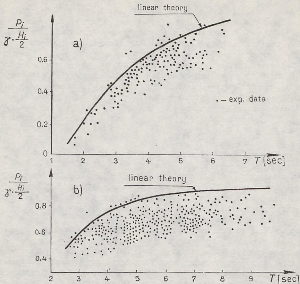
Fig. 2. Attenuation of particular sea surface oscillations, [13]; a) deep water; b) shallow water
