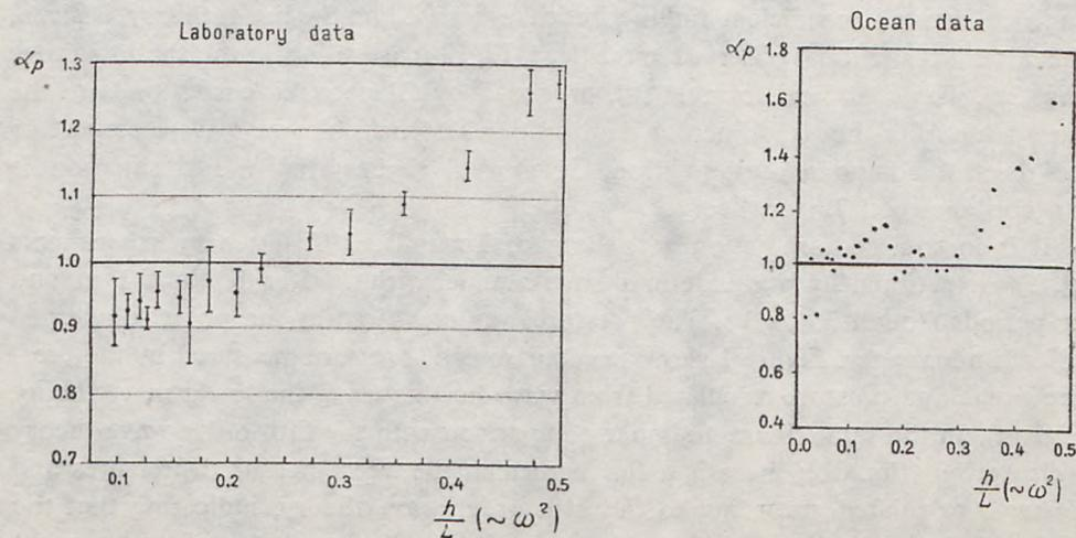
Fig. 3. Experimental damping coefficient  $\alpha_p$  for laboratory and ocean data, [14]
