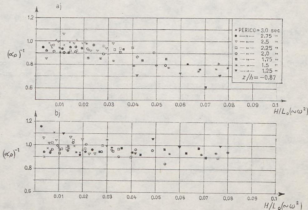
Fig. 1. Experimental and theoretical attenuation of wave pressure [2] a) according to linear theory; b) according to 5th order theory
