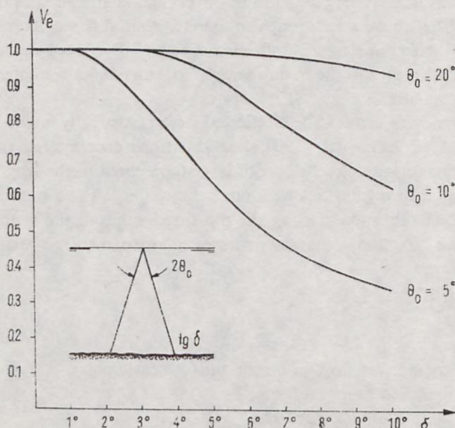
Fig. 1. Dependence of the measured coefficient of reflection from the bottom on the directional characteristics of the transmitting-receiving transducer and the inclination angle of irregularities of reflecting surface
