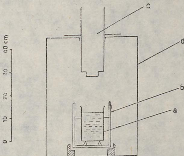
Fig. 1. Schematic diagram of the measuring chamber with photometer used in bioluminescence studies: *a* — measuring tray with sample; *b* — mirror shield with thermostable bath; *c* — photometer; *d* — light-proof chamber
