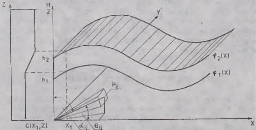
Fig. 1. Schematic diagram of the sound velocity distribution in the sea in the presence of an internal wave.
