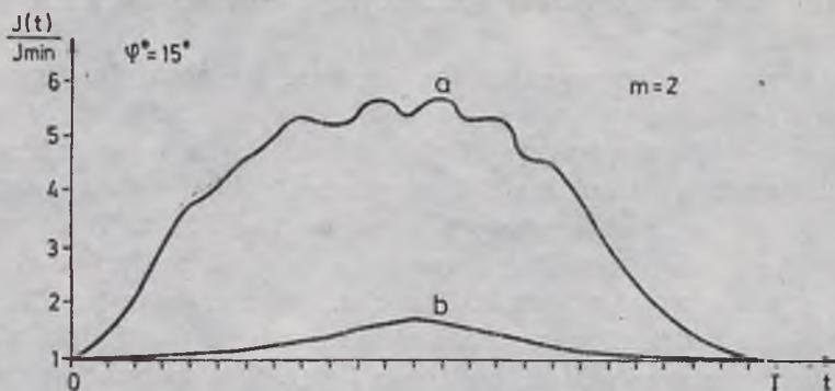
Fig. 3. Relative variations of the noise intensity below the internal wave for summer (a) and winter (b) sound velocity profiles.
