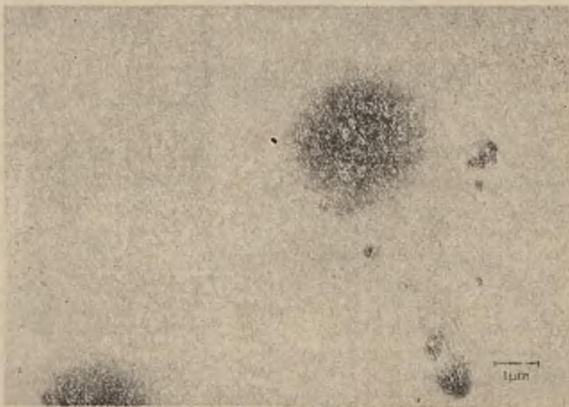
Fig. 4. Microphotograph of standard mercury particles deposited on metallic gold foil at a 7300-fold magnification.
