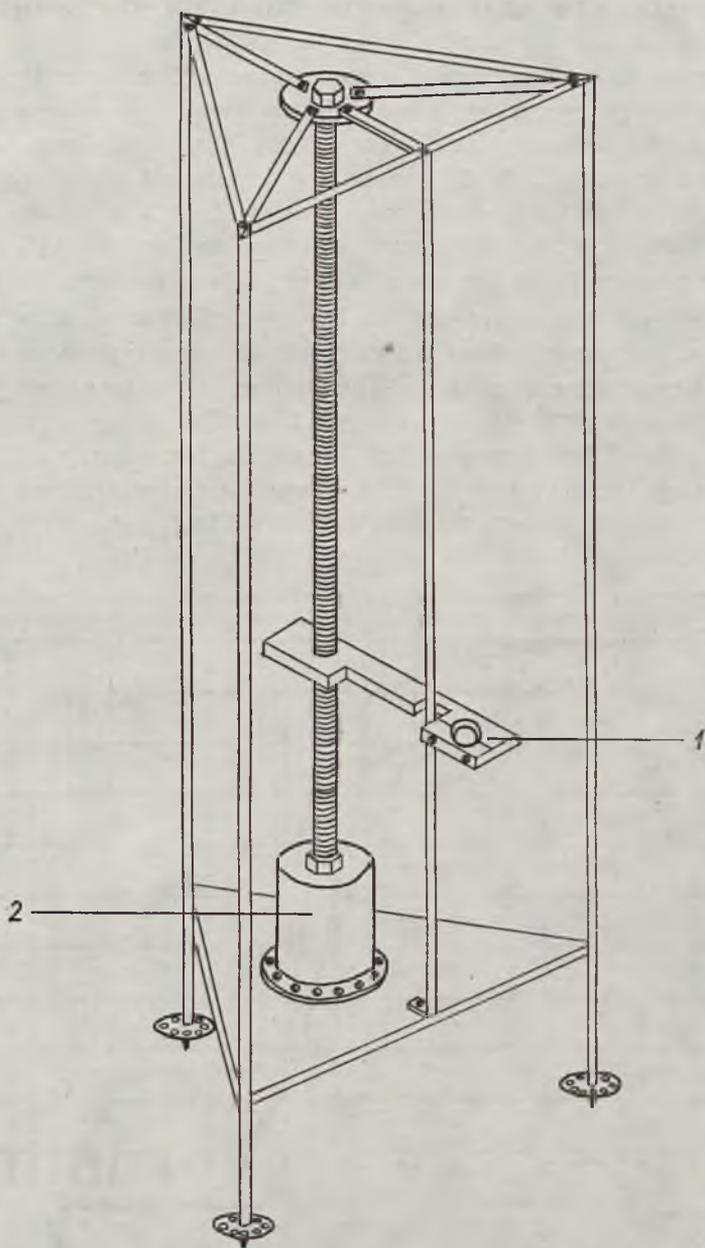
Fig. 3. Schematic diagram of hydrophone structure
