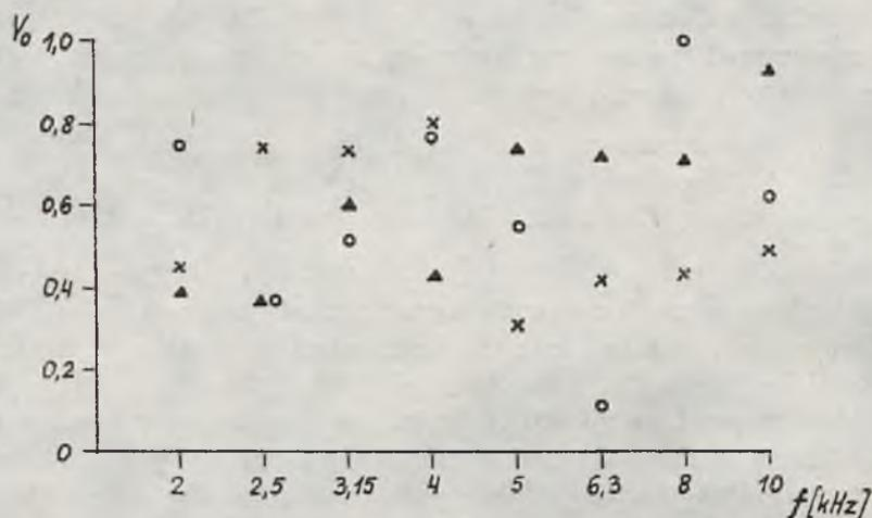
Fig. 5. Absolute value of reflectivity,  $V_0$ , versus frequency of acoustic wave  $f(\vartheta = 0^\circ)$
