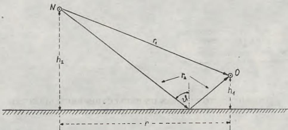
Fig. 1. Configuration of transmitter (N) and receiver (O) for the incidence angle of an acoustic wave on the bottom  $\vartheta \neq 0^\circ$
