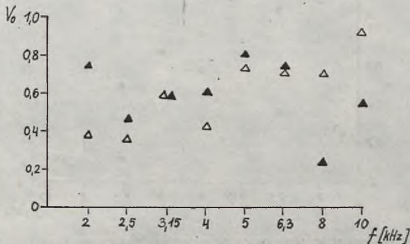
Fig. 8. Experimental absolute values of reflectivity for very fine sand, versus frequency of acoustic wave, at two angles of incidence
