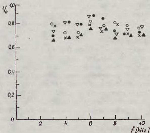
Fig. 6. Experimental absolute values of sea-floor reflectivity,  $V_0$ , versus frequency. Different notations correspond to various measuring points. According to Grubnik [2]
