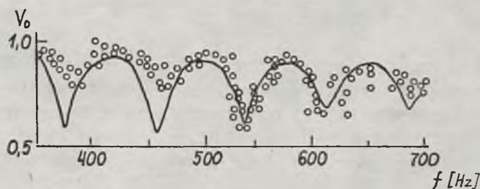
Fig. 7. Absolute value of reflectivity versus frequency for a two-layer model of the sea floor (the case  $C_2 \ll C_0$ , in which  $C_2$ ,  $C_0$  — speeds of sound in the upper layer and in water, respectively). According to Goncharenko, Zakharov, Ivanov, Kirshov [3]
