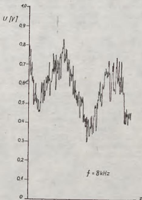
Fig. 10. Examples of recorded interference fields, obtained when the hydrophone moved along the z-axis (vertical axis oriented upwards from the bottom). The drawings correspond to various frequencies of acoustic waves
