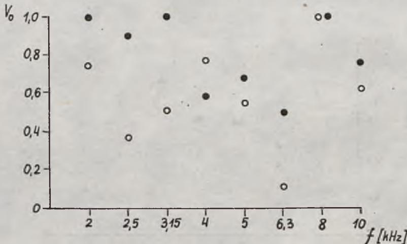
Fig. 9. Experimental absolute values of reflectivity from a sea floor consisting of macrofauna (molluscs, snails), versus frequency of acoustic wave, for two angles of incidence
