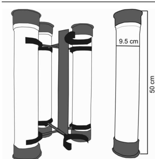
**Figure 2.** Sediment traps – side view
