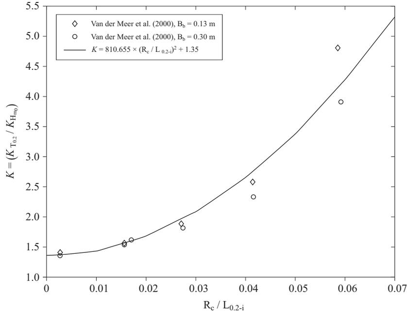
**Figure 10.** Data fitting of equation (7), for an emerged smooth breakwater, with coefficient  $A$  independent of parameter  $R_c/H_{m0}$  and coefficient  $B = 1.35$
