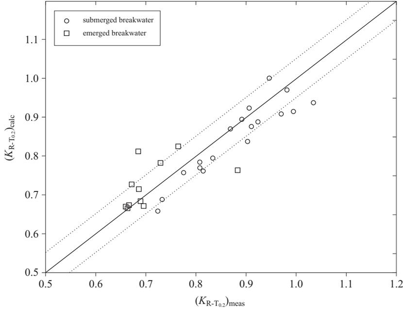
**Figure 11.** Diagram comparing the measured reduction coefficients of the mean spectral wave period  $(K_{R-T_{0.2}})_{meas}$  and the values calculated by means of equation (10) and equation (11)  $(K_{R-T_{0.2}})_{calc}$  for submerged and emerged breakwaters
