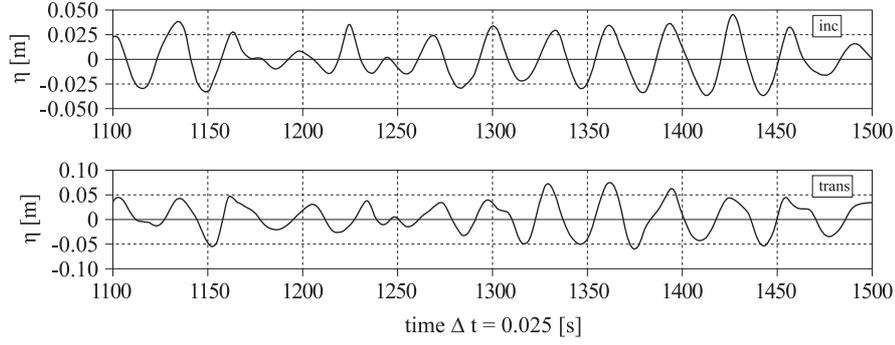
**Figure 3.** Incident and transmitted wave time series for raw data recorded on gauge G1 (inc) and gauge G4 (trans), (Test 2, Table 1)
