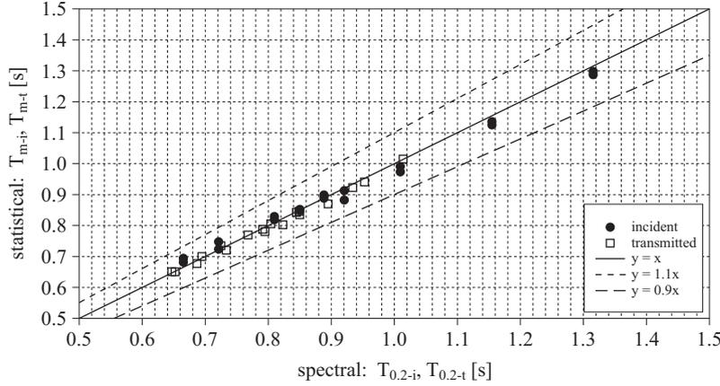
**Figure 6.** Ratio of spectral ( $T_{0.2}$ ) and statistical ( $T_m$ ) mean wave periods for incident and transmitted waves at a smooth submerged breakwater
