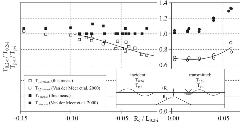
**Figure 7.** Dependence of parameters  $T_{0.2-t}/T_{0.2-i}$  and  $T_{p-t}/T_{p-i}$  on relative submersion  $R_c/L_{0.2-i}$ , for a smooth breakwater with submerged crown (from this paper) and an emerged crown as per Van der Meer's (Van der Meer et al. 2000) measurements with crown width  $B_b = 0.13$  and  $0.3$  m;  $H_{m_0} = 0.09-0.14$  m, wave steepness  $s_{op} = 0.03$ , water depth  $d = 0.29-0.37$  m, breakwater slope 1:4,  $R_c/H_{m_0} = 0-1.0$
