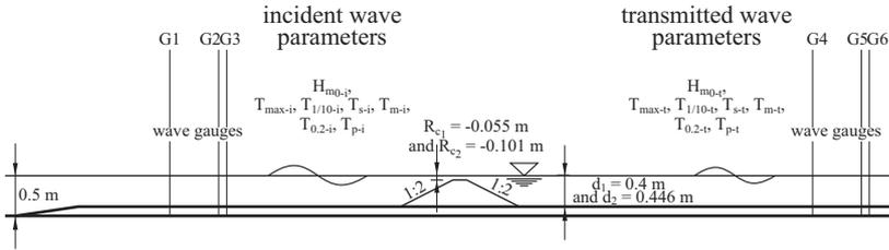
**Figure 1.** Details of the wave flume and measured incident and transmitted wave parameters
