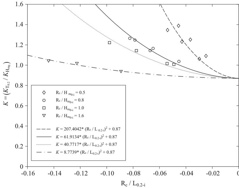
**Figure 9.** Data fitting of equation (7), for four categories of parameter  $R_c/H_{m_{0-i}} = 0.5, 0.8, 1.0$  and  $1.6$ , for a submerged smooth breakwater, coefficient  $B = 0.87$
