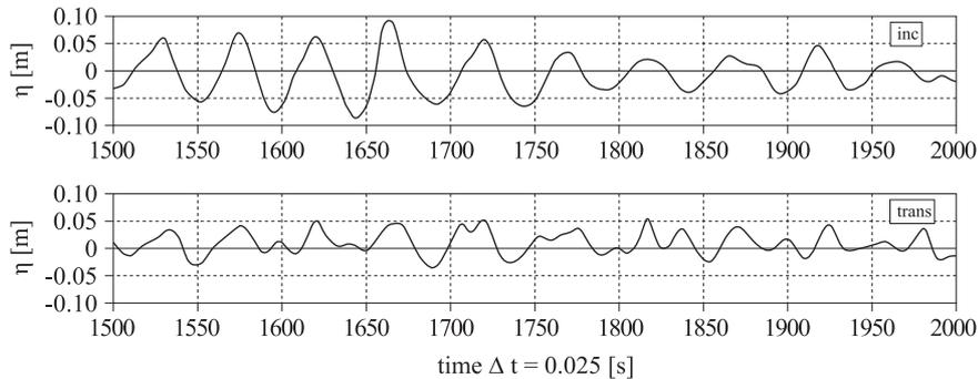
**Figure 2.** Incident and transmitted wave time series for raw data recorded on gauge G1 (inc) and gauge G4 (trans), (Test 8, Table 1)
