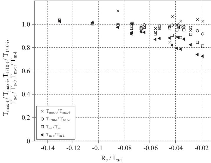
**Figure 4.** Reduction in statistical wave periods crossing a smooth submerged breakwater;  $T_{\max-i}$ ,  $T_{1/10-i}$ ,  $T_{s-i}$ ,  $T_{m-i}$  – incident wave periods;  $T_{\max-t}$ ,  $T_{1/10-t}$ ,  $T_{s-t}$ ,  $T_{m-t}$  – transmitted wave periods
