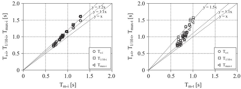
**Figure 5.** Ratio of statistical wave periods  $T_{\max-i}$ ,  $T_{1/10-i}$  and  $T_{s-i}$  in front of (left) and  $T_{\max-t}$ ,  $T_{1/10-t}$  and  $T_{s-t}$  behind (right) a smooth submerged breakwater with mean statistical periods  $T_{m-i}$  and  $T_{m-t}$  (ordinate-y, abscissa-x)
