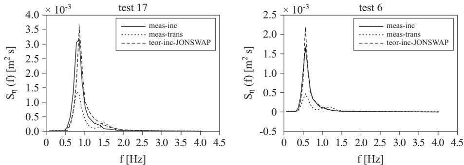
**Figure 8.** Comparison of the measured incident, theoretical incident (JONSWAP) and transmitted spectra for tests 17 and 6
