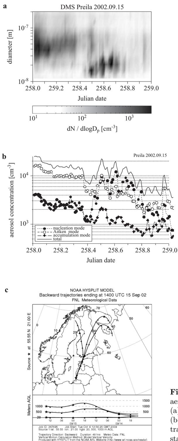
**Figure 3.** Time evolution of aerosol particle size distribution (a), modal aerosol concentration (b) and backward air mass trajectories (c) at the Preila station on 15 September 2002
