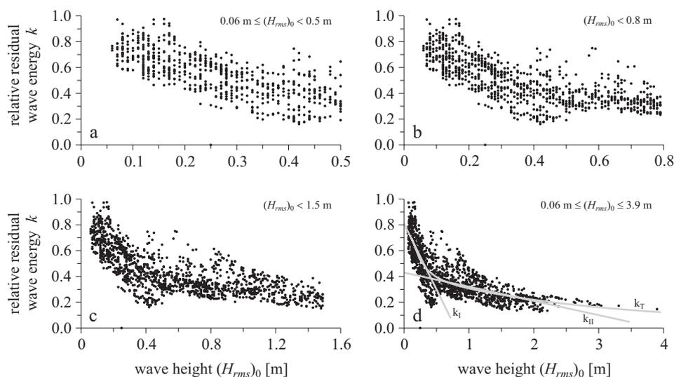
**Figure 7.** Relative residual wave energy  $k = f((H_{rms})_0)$  at depth  $h \approx 0.5$  m for various ranges of incident wave height  $(H_{rms})_0$
