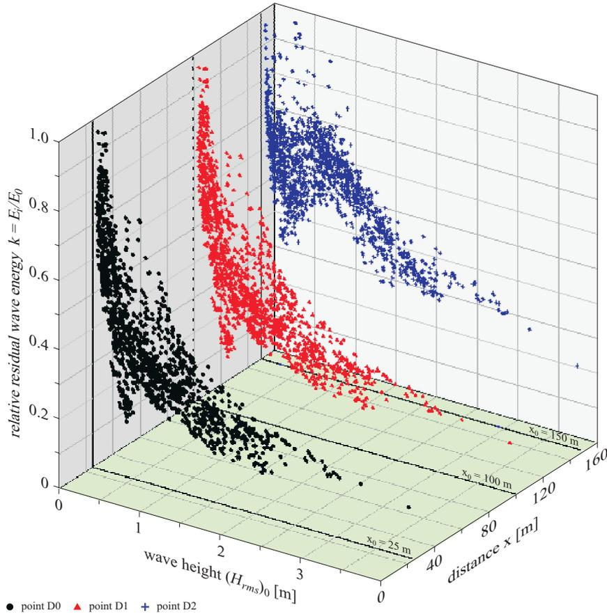
**Figure 6.** Wave energy dissipation  $k$  as a function of distance from the shoreline  $x$  and deep-water wave height  $(H_{rms})_0$
