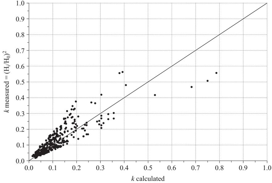
**Figure 8.** Comparison of experimental values of relative wave energy  $k$  with theoretical results from eq. (8)
