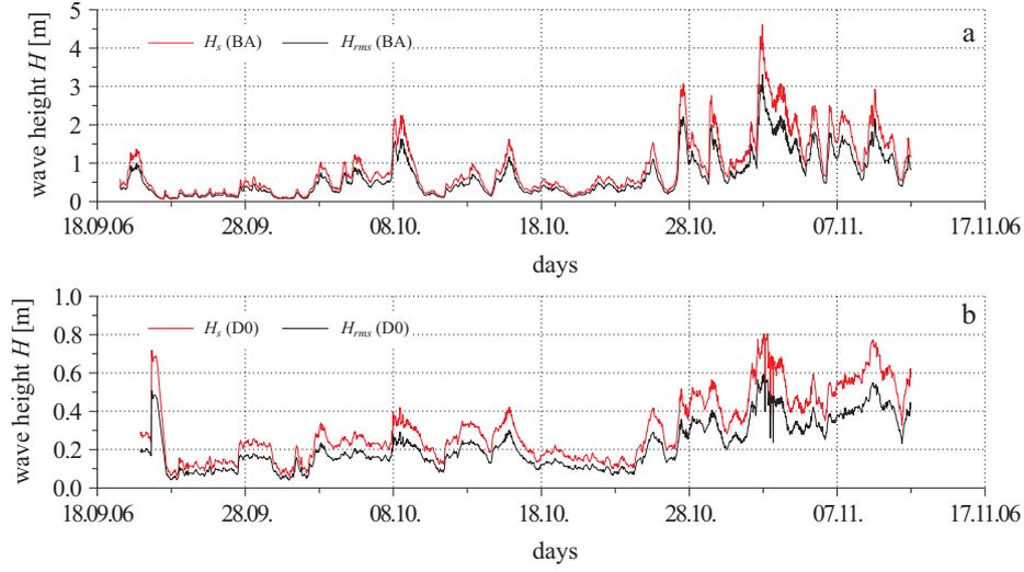
**Figure 5.** Wave height series  $H_s$  and  $H_{rms}$  recorded at offshore (a) and nearshore (b) locations
