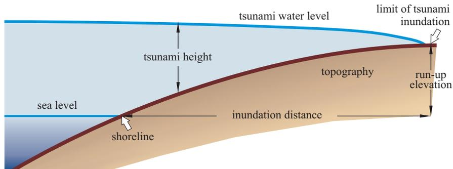
**Fig. 3.** Measurement of inundation distances and run-up elevation (method adopted from USGS survey team – weblinks)
