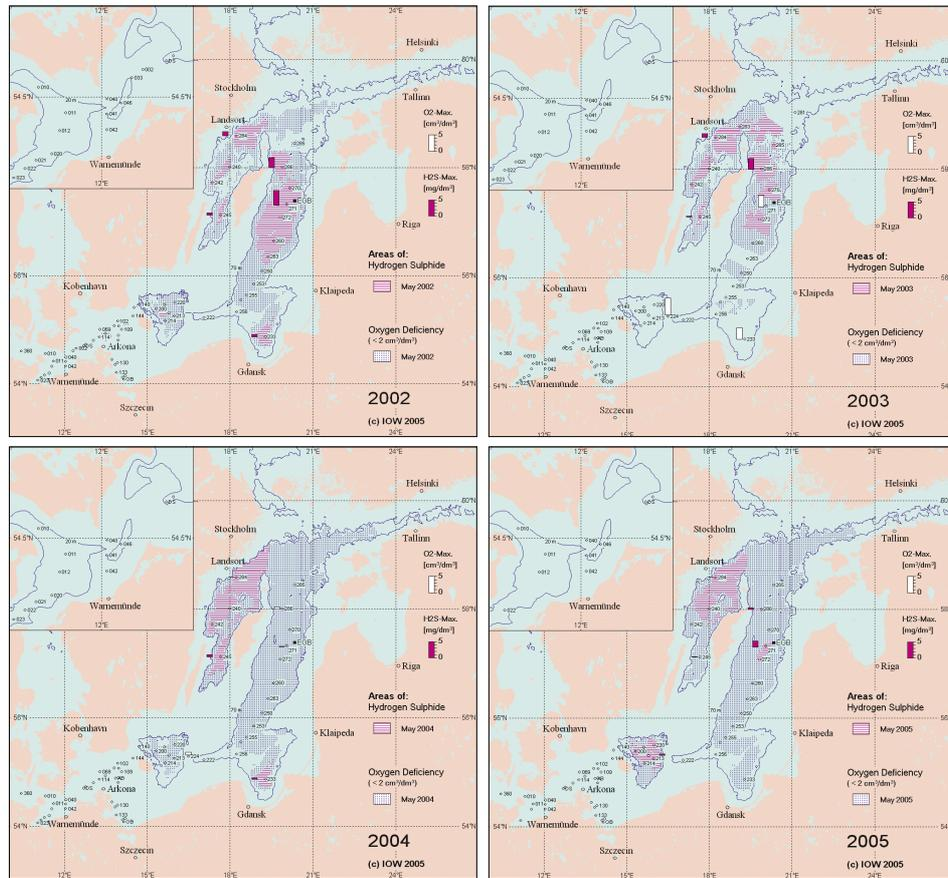
**Fig. 4.** Near-bottom distributions of oxygen and hydrogen sulphide concentrations for the months of May in 2002–2005. The inset in the top left-hand corner magnifies the western Baltic
