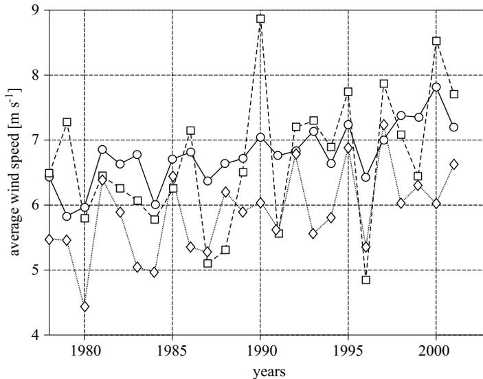
**Fig. 9.** The annual average wind speed (circles on solid line) and average wind speed at Utö in March (squares on dashed line) and April (diamonds on dotted line) 1978–2001
