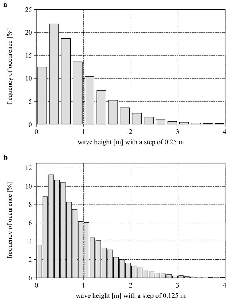
**Fig. 3.** Frequency of occurrence of wave heights at Almagrundet 1978–95 according to the SimRad wave data 1978–96 for wave height steps of 0.25 m (a) and 0.125 m (b)
