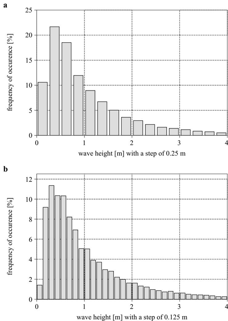
**Fig. 4.** Frequency of occurrence of wave heights at Almagrundet 1993–2003 according to the WHM wave data 1993–2003 for wave height steps of 0.25 m (a) and 0.125 m (b)
