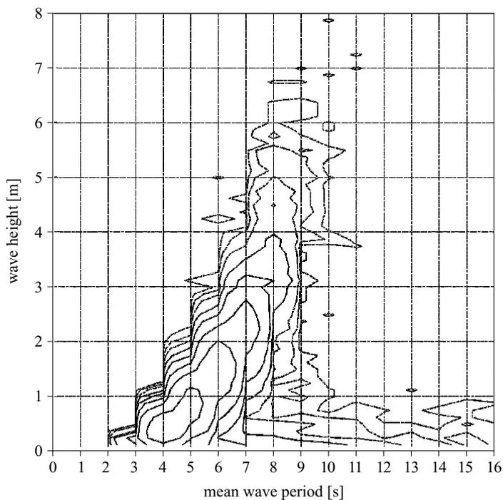
**Fig. 5.** Scatter diagram of wave heights  $H_{1/3}$  and mean periods in the SimRad data. The wave height step is 0.125 m. The range of periods is shown on the horizontal axis: for example, 2 s stands for  $T_z < 2.5$  s, 3 s stands for  $2.5 \leq T_z < 3.5$  s etc. Isolines for 1, 3, 10, 33, 100, 330, 1000 and 3300 cases are plotted, whereas isolines for 1–10 cases are dashed lines
