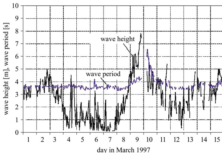
**Fig. 7.** The wave height  $H_{1/3}$  and the mean period at Almagrundet in March 1997 according to the WHM data
