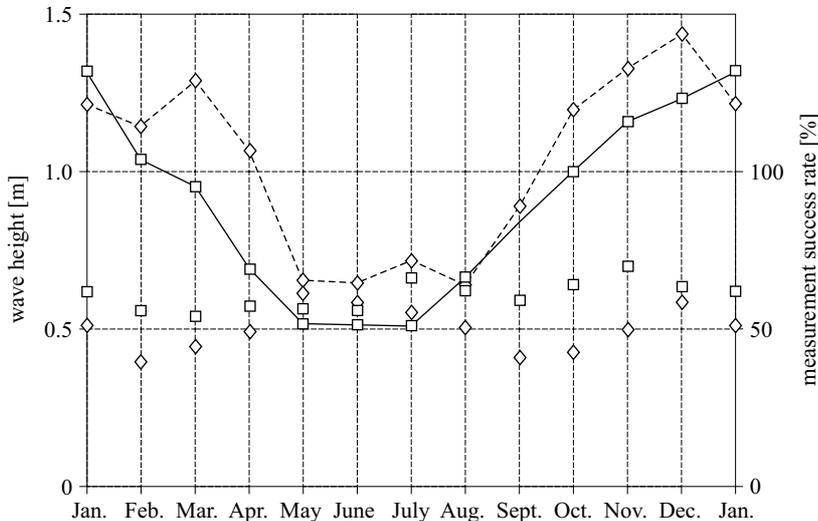
**Fig. 10.** The monthly mean wave height measured by the SimRad (squares on solid line) and the WHM (diamonds on dashed line) equipment. The measurement success rate (separated squares and diamonds) is the percentage of acceptable measurements within a particular month
