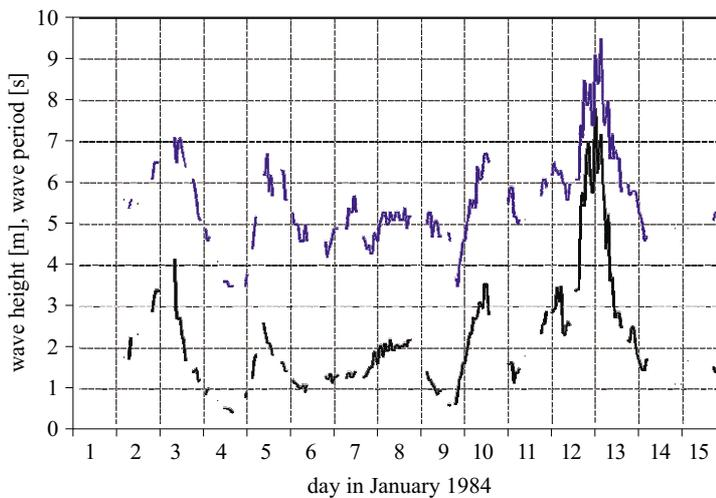
**Fig. 6.** The wave height  $H_{1/3}$  (lower line) and the mean period (upper line) at Almagrundet in January 1984 according to the SimRad data. Note the large numbers of gaps in the lines, which correspond to the missing data
