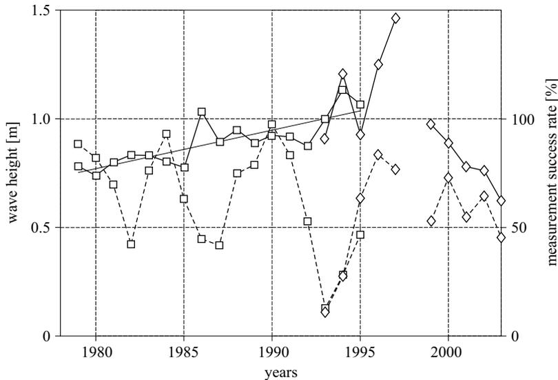
**Fig. 8.** The annual mean wave height  $H_{1/3}$  measured by the SimRad equipment (squares on solid line), the relevant trend line for the years 1979–95, and the wave height measured by the WHM equipment (diamonds on solid line). The measurement success rate (squares and diamonds on dashed lines) is the percentage of acceptable measurements within a particular year
