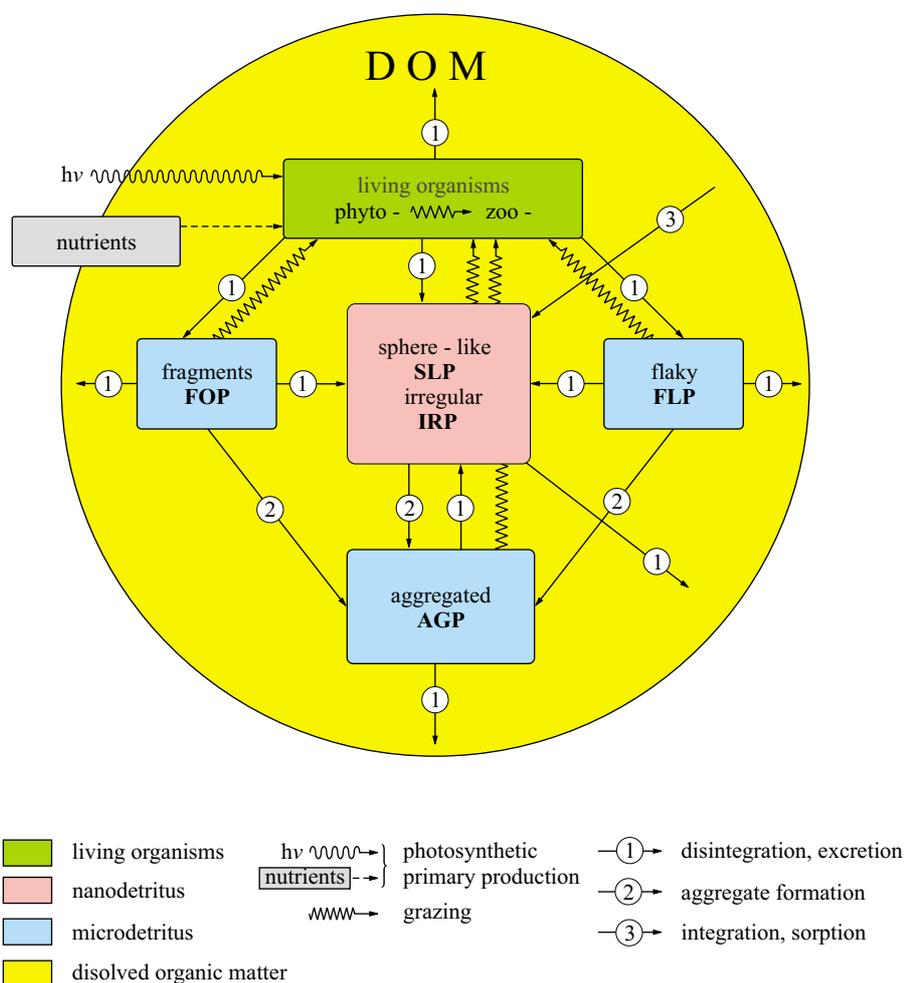
**Fig. 2.** Simplified scheme of the formation and evolution of the various morphological groups of POM
