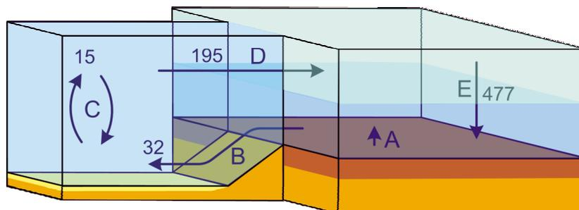
**Fig. 9.** A sketch of the phosphorus cycle in the northern Little Belt based on net calculations of one year of data. The process components of the phosphorus cycle are: A: Nutrient release, B: Advection, C: Mixing, D: Advection (also in the form of transport of algae) and E: settling and deposition (sedimentation data from Christiansen et al. 1997). Numbers on the sketch are in tonnes P per year
