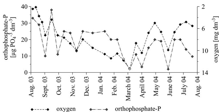
**Fig. 6.** Orthophosphate-P and oxygen concentrations near the bottom of the water column at NLB51. Note that the oxygen axis is inverted
