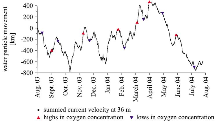
**Fig. 8.** Summed particle travel distance at 36 m water depth measured with an ADCP at the old Little Belt Bridge station. Increasing values result from outflow and decreasing values from inflow. Highs and lows in oxygen concentration near the bottom of NLB51 are also shown
