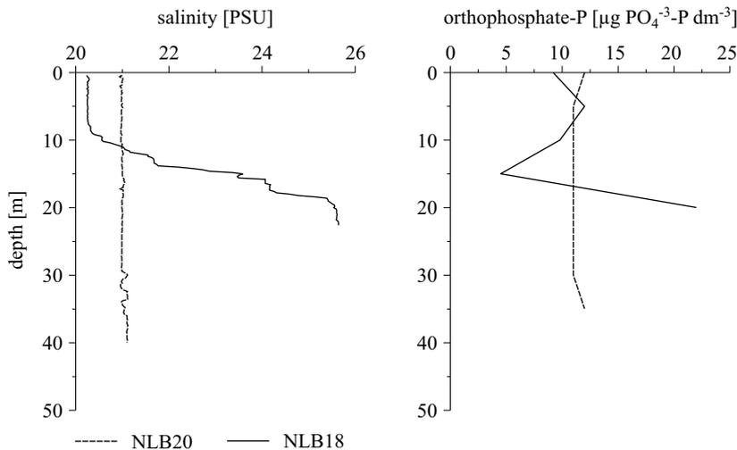
**Fig. 7.** Salinity and orthophosphate-P profiles on February 23, 2004 at NLB18, a stratified station, and at NLB20, a mixed station
