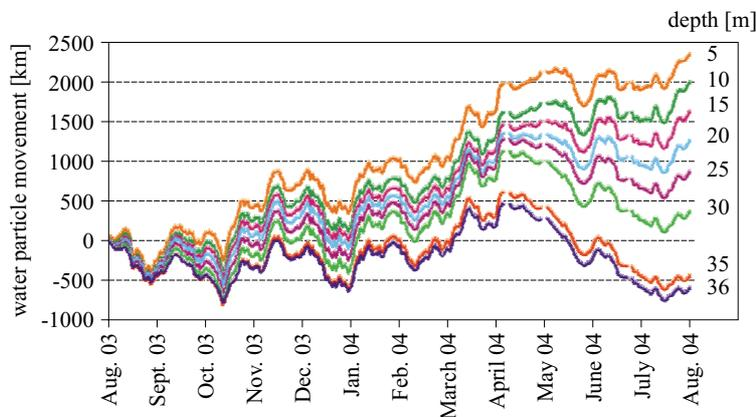
**Fig. 3.** Summed current velocity measured with an ADCP at 8 different water depths obtained at the old Little Belt Bridge showing the flow distance of a water particle during the campaign, assuming that the velocity remains the same as that measured at the bridge
