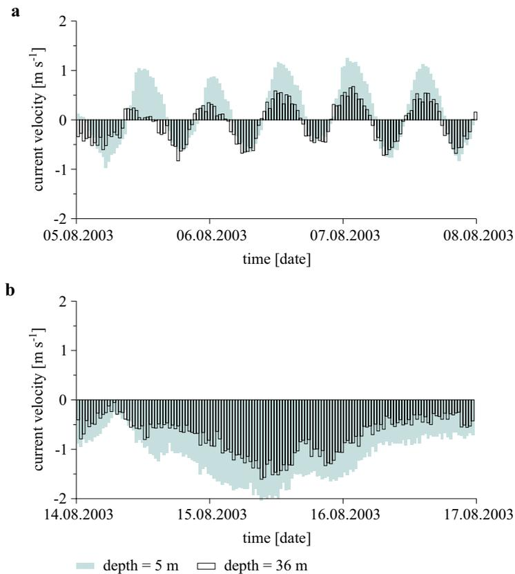
**Fig. 2.** Current velocities at 5 and 36 m depth obtained at the old Little Belt Bridge measured with an ADCP. Northward (outflow) current velocity is marked as positive values, and southward (inflow) velocity is negative. Current velocity varying with the tide (a). Current velocity during a westerly wind episode with wind speeds around 13 m s<sup>-1</sup> (b)
