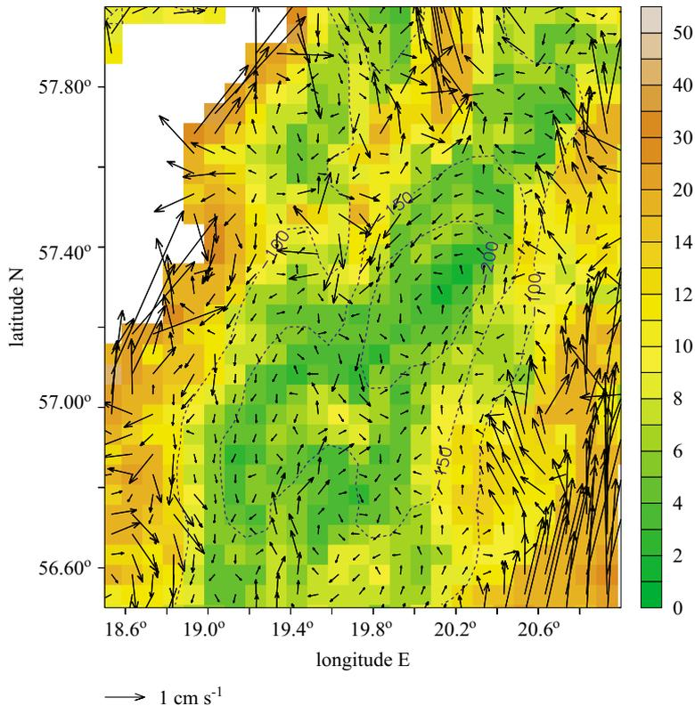
**Fig. 7.** Maximum near-bottom current velocities [ $\text{cm s}^{-1}$ ] as derived from a 3-D model for the simulation period 1970–1993. The main bathymetry is indicated by dashed isolines for 100, 150 and 200 m depth
