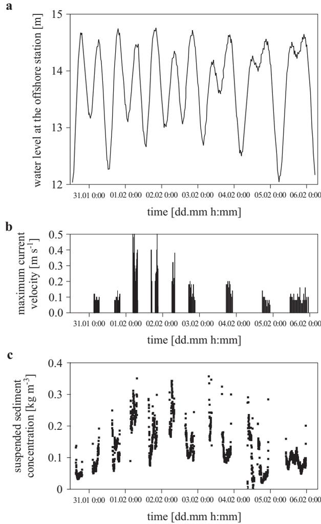
**Fig. 6.** Suspended sediment concentration during a 6-day experiment. Water level at the offshore station in the Dong Tranh estuary (a); maximum current velocity at ST2 (b); suspended sediment concentration at ST2 (c)
