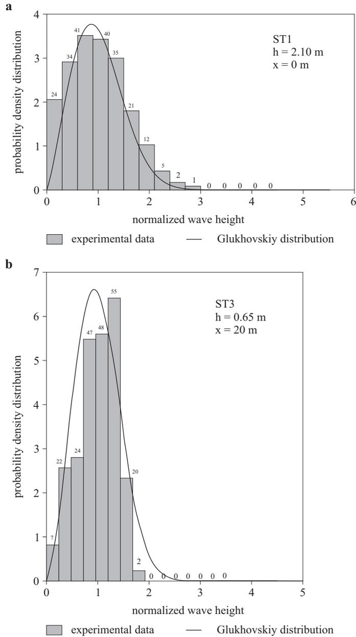
**Fig. 4.** Comparison of the Glukhovskiy's probability density function for wave height with experimental data at ST1 (a) and ST3 (b) on 01 February 2005 at 19:00
