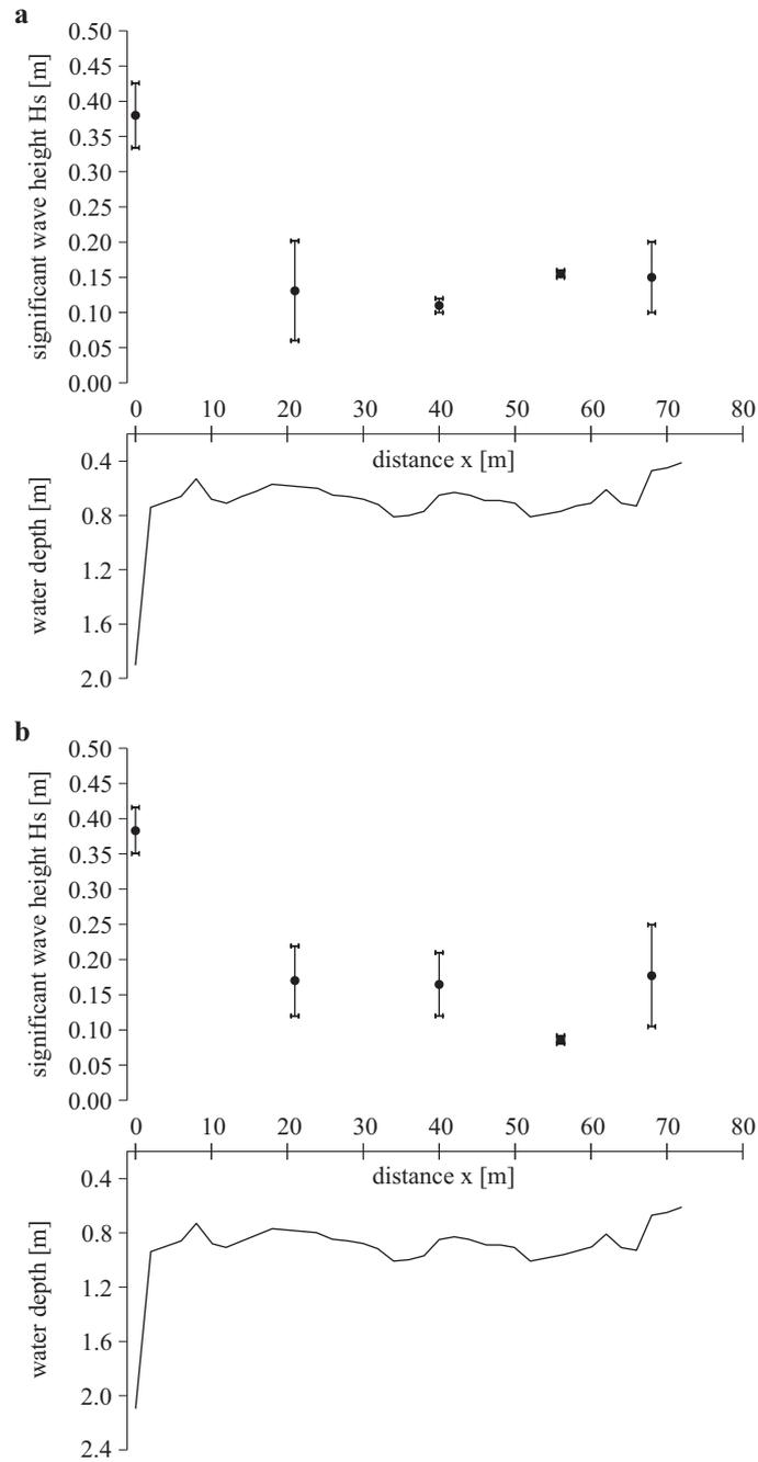
**Fig. 3.** Experimental wave height attenuation with varying water depth at the Nang Hai mangrove site:  $h = 1.90$  m (a),  $h = 2.10$  m (b),  $h = 2.5$  m (c). The filled circles denote mean values and the horizontal bars indicate the range of wave height changes
