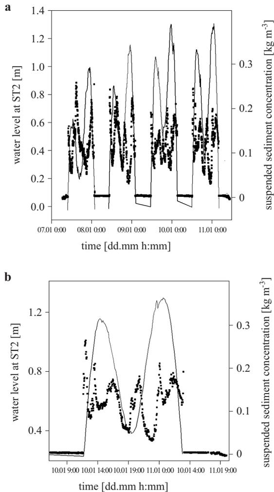
**Fig. 8.** Suspended sediment concentration for the high wave case: high spring tide in January 2005 (a), one tidal cycle (b)
