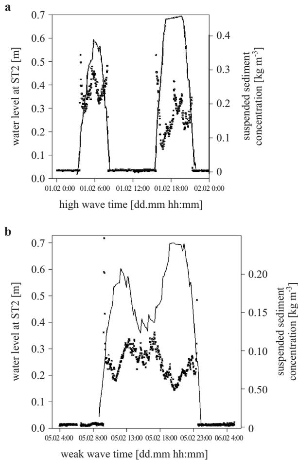
**Fig. 7.** Comparison of suspended sediment concentration in one tidal cycle in the case of high waves (a) and weak waves (b)
