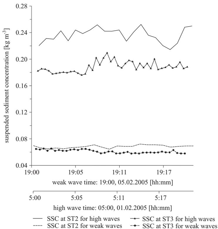
**Fig. 9.** Comparison of suspended sediment concentrations at ST2 and ST3 in the case of weak and high wave action
