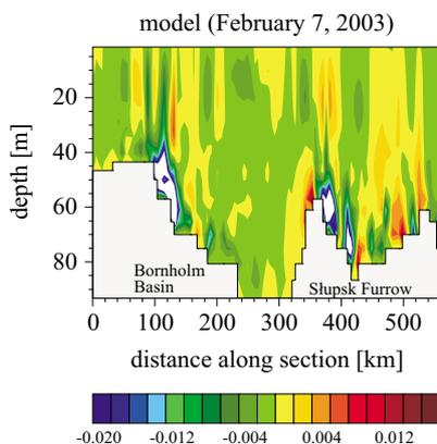
**Fig. 12.** Cross-section of simulated vertical velocity (in  $\text{cm s}^{-1}$ ) from the Bornholm Channel to the Słupsk Furrow on February 7, 2003. The position of the section is depicted in Fig. 1. Velocities smaller than  $-0.02 \text{ cm s}^{-1}$  are shown in white
