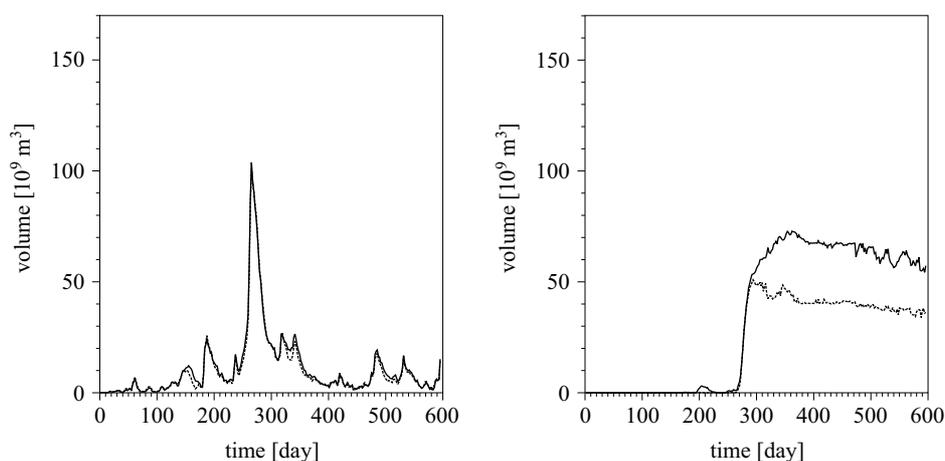
**Fig. 7.** Volume (in  $\text{km}^3$ ) of highly saline water ( $S > 17 \text{ PSU}$ ) in the Arkona Basin (left) and the Bornholm Basin (right) during the 2003 inflow event: reference run (solid line), experiment without BBL (dotted line). The time axis starts on May 1, 2002
