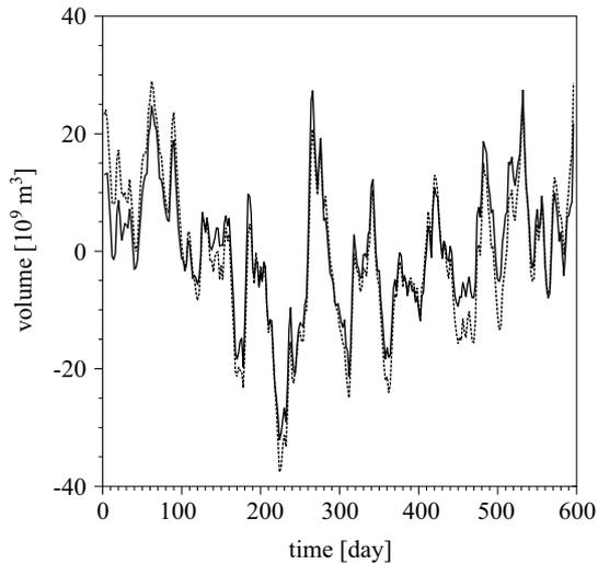
**Fig. 3.** 2-daily detrended accumulated inflow (in  $10^9 \text{ m}^3$ ) through the Sound: RCO (solid), hydraulic model by Håkansson (2004) (dotted). The time axis starts on May 1, 2002
