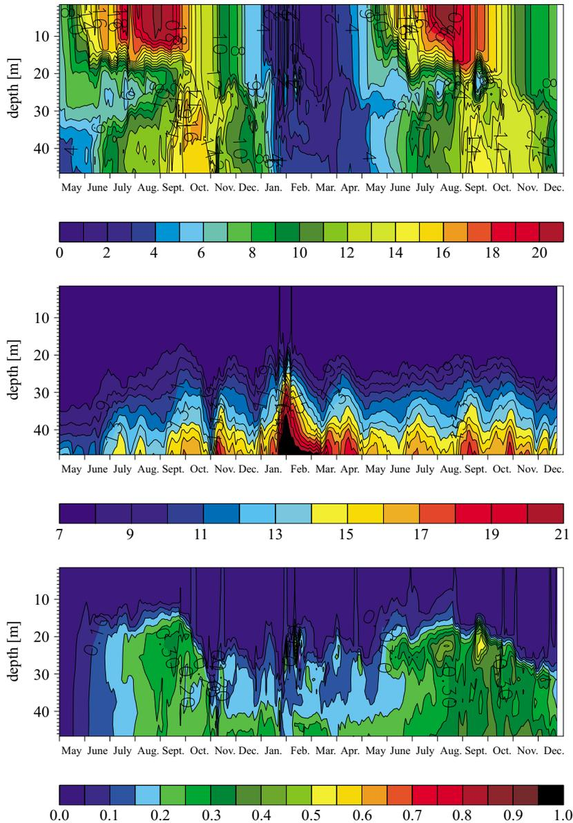
**Fig. 9.** Simulated temperature (in °C, upper panel), salinity (in PSU, middle panel), and age (in years, lower panel) as a function of time and depth in the Arkona Deep (BY2, see Fig. 1; cf. Feistel et al. (2003b), their Fig. 3). The time interval May 2002 to December 2003 is shown
