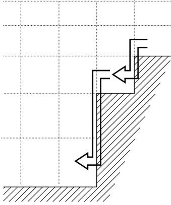
**Fig. 13.** BBL connecting bottom boxes of the OGCM, enabling advective or diffusive transports along the bottom. (Figure taken from Döscher & Beckmann 2000)
