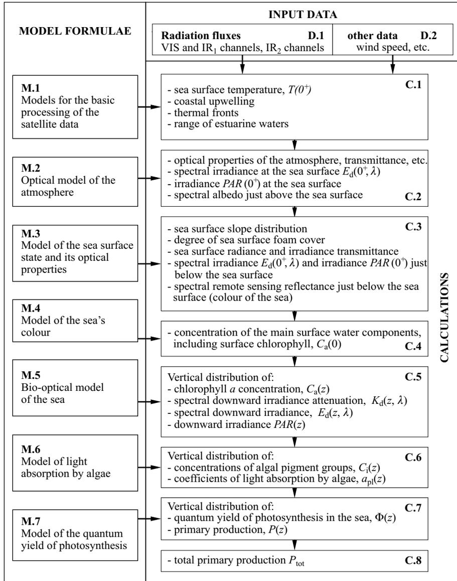
**Fig. 1.** Block diagram of the DESAMBEM algorithm
