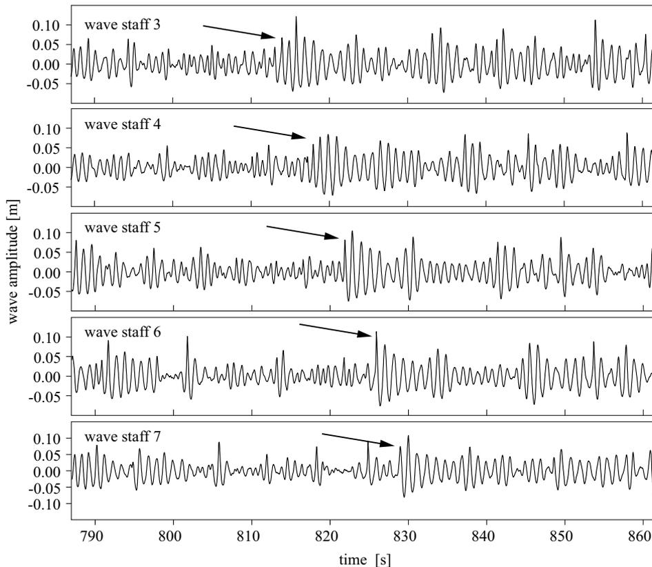
**Fig. 5.** Surface wave variation recorded by 5 consecutive wave staffs. The arrows indicate the time evolution of the breaking event
