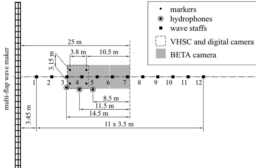
**Fig. 1.** Experimental set-up
