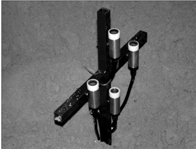
**Fig. 5a.** Pore pressure gauge system
