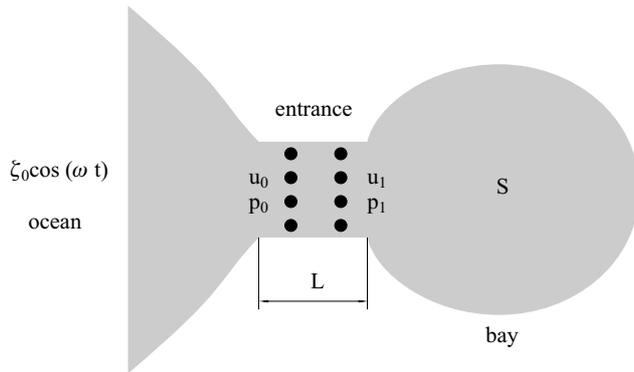
**Fig. 20.** Diagram of tidal power construction and hydrodynamic modeling in a bay. On the ocean side the tide is described by  $\zeta_0 \cos(\omega t)$ , the dots depict the tidal current generators located in the entrance to the bay
