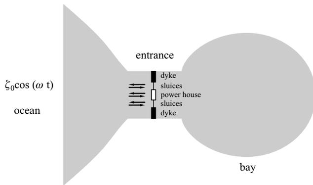
**Fig. 15.** Tidal power plant constructed at the entrance to a single bay
