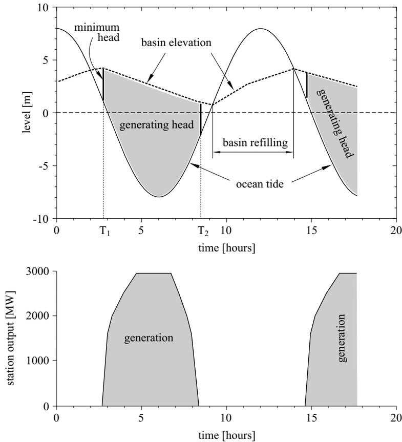
**Fig. 16.** Tidal power generation: typical one-way cycle for a single bay. Upper panel, sea level inside and outside the bay. Lower panel, power output in time
