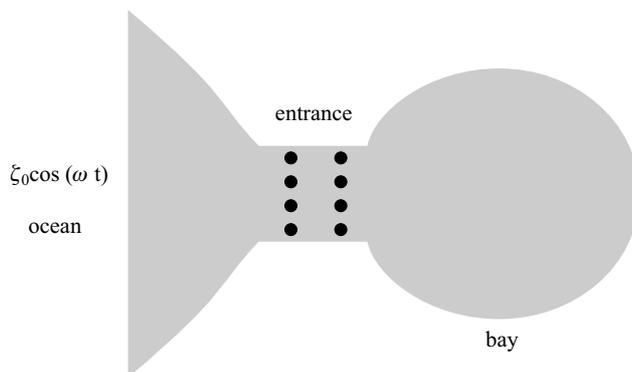
**Fig. 14.** Diagram of a TPP and hydrodynamical modeling in a bay with a large tidal range. In the ocean the tide is described by  $\zeta_0 \cos(\omega t)$ , the dots represent a tidal barrage or tidal current generators
