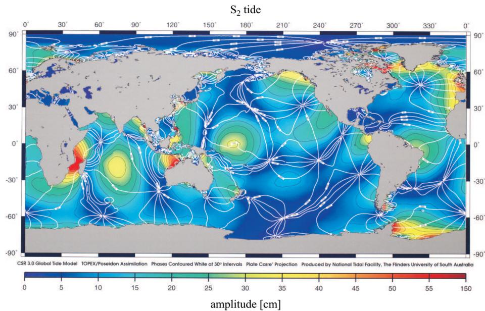
**Fig. 2.** S<sub>2</sub> tide in the World Ocean. Amplitude (dark lines) is given in cm and phase (white lines, degree) is referred to Greenwich. Courtesy of G. Musiela, NTF, Australia
