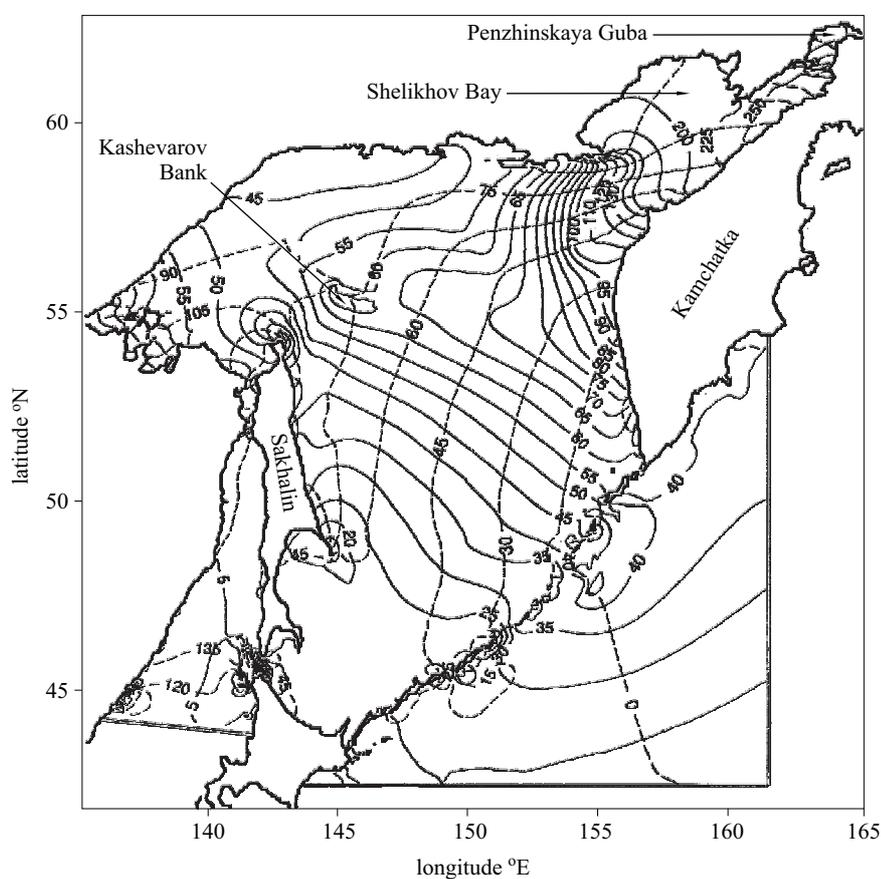
**Fig. 6.** Amplitude and phase of the  $K_1$  tide in the Okhotsk Sea based on Kowalik & Polyakov (1998). The amplitude (solid lines) is in cm and the phase (dashed lines, degree) is referred to Greenwich
