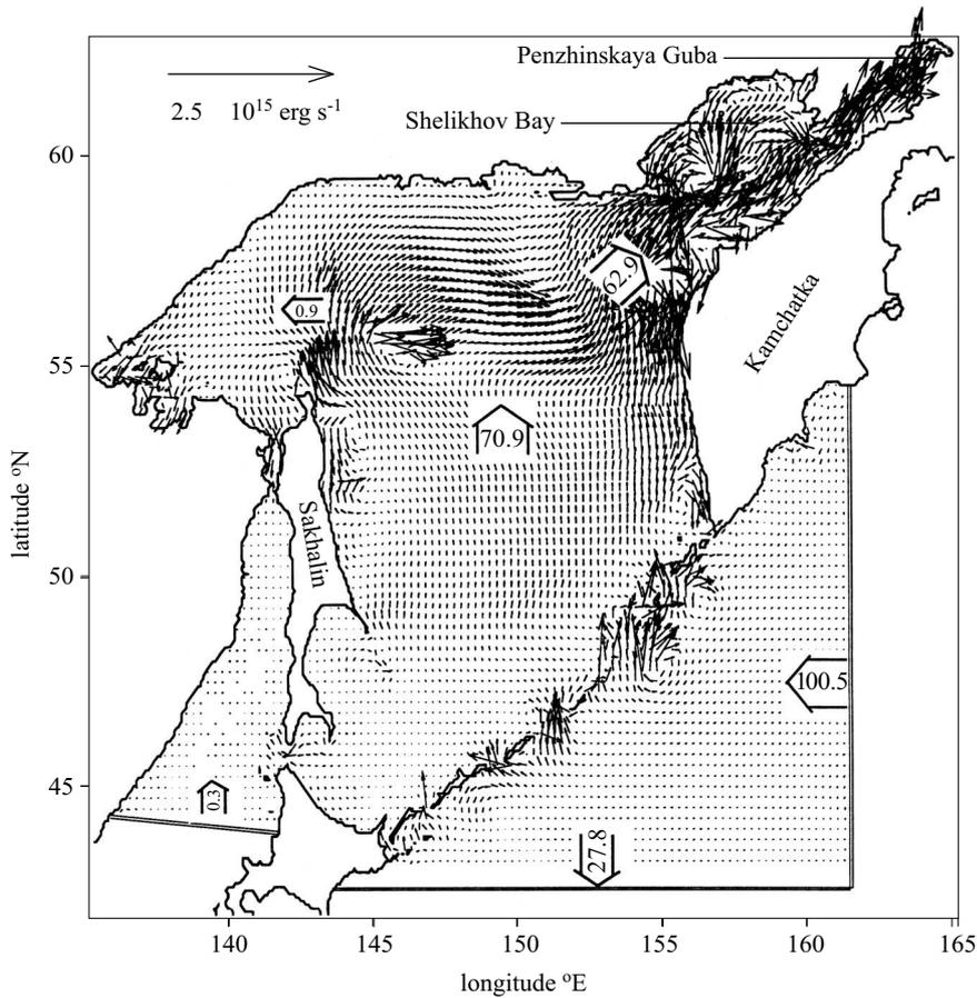
**Fig. 12.** Tidal energy flux for  $K_1$  tide in the Sea of Okhotsk based on Kowalik & Polyakov (1998). The large arrows show the net energy flux across transects. The values inside the arrows should be multiplied by  $10^{16} \text{ erg s}^{-1}$
