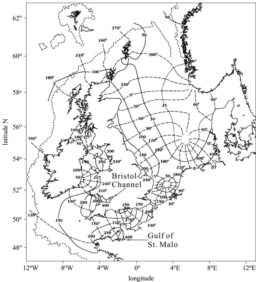
**Fig. 9.** Amplitude and phase of the  $M_2$  tide in the north-west European Shelf Seas, based on Flather (1976). The amplitude (solid lines) is in cm and the phase (dashed lines, degree) is referred to Greenwich
