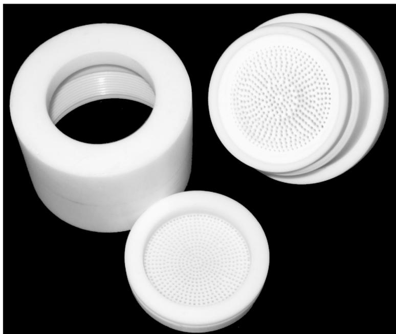
**Fig. 1.** Filter pack for aerosol collection used in the tests and measurements
