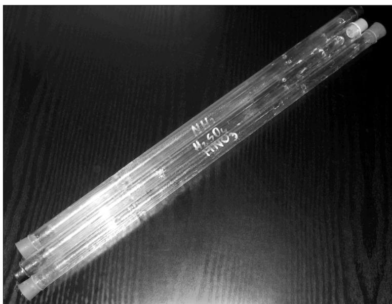
**Fig. 2.** Denuders for gaseous ammonia collection used in the tests and measurements
