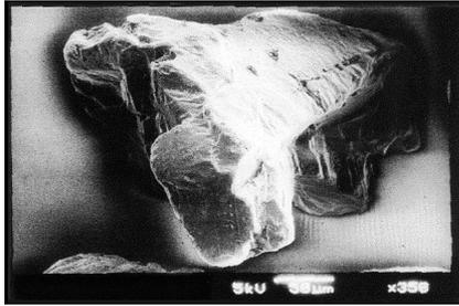
**Plate 3.** Subrounded quartz grains showing conchoidal fracture with V marks
