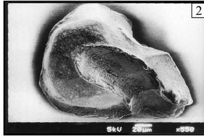
**Plate 1 and Plate 2.** Quartz grain showing conchoidal fracture with cavities and solution pitting
