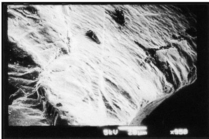
**Plate 5.** Quartz grain with solution pits and silica precipitation patterns
