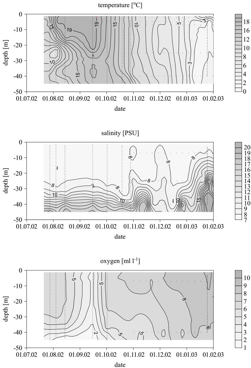
**Fig. 3.** Vertical profiles of temperature, salinity and oxygen concentration recorded by the Arkona Basin buoy (after September 2002) combined with ship-borne CTD measurements for the period 27th July 2002 – 1st February 2003. The dots indicate measured samples. The warm inflow period peaked in mid-September 2002 and coincided with a significant oxygen deficiency throughout the water column
