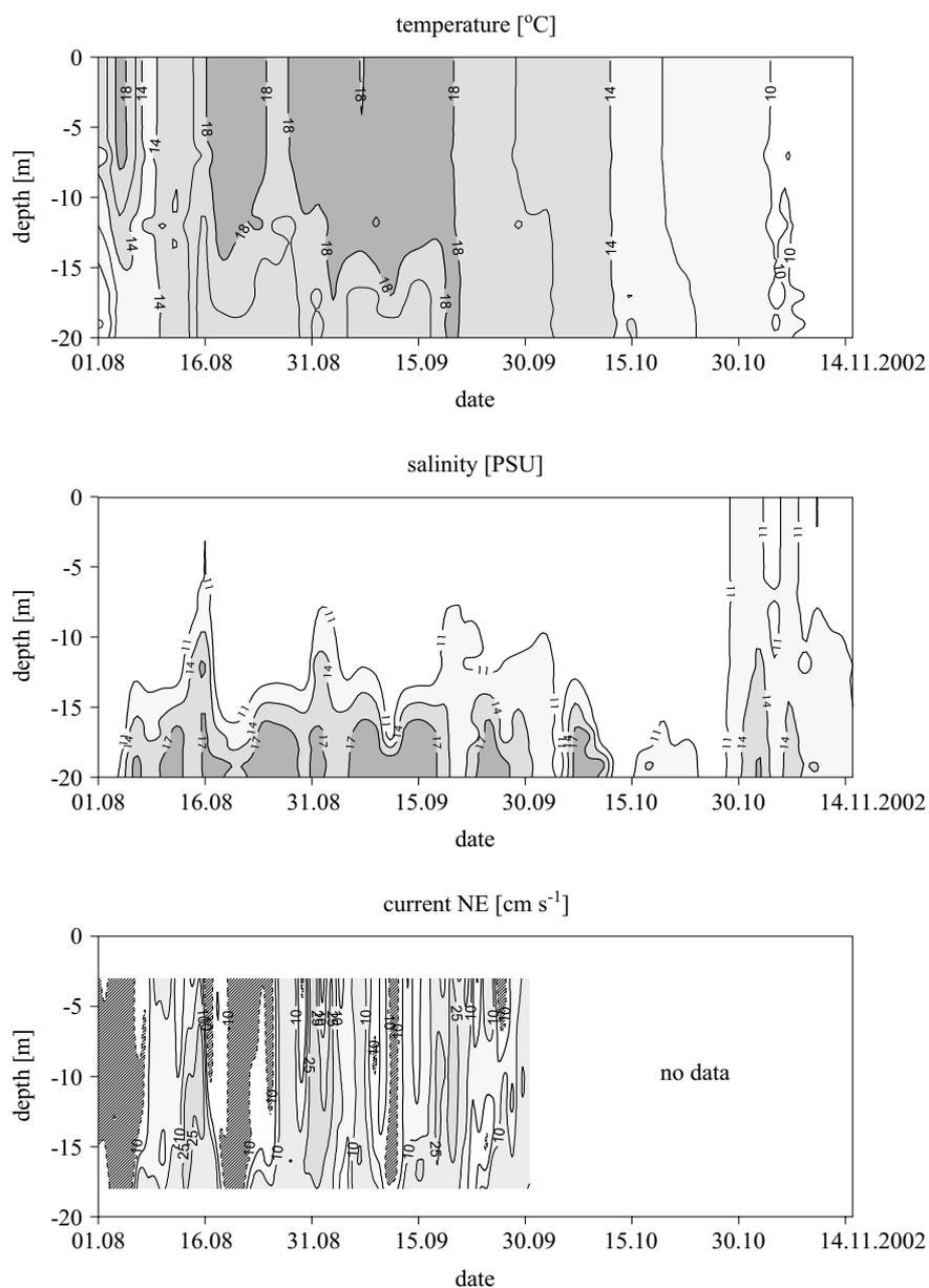
**Fig. 2.** Vertical profiles of temperature, salinity and north-easterly current component at the Darss Sill measuring mast between 1st August 2002 and 14th November 2002. Note especially the strong salinity stratification as opposed to the almost homogeneous vertical current profiles
