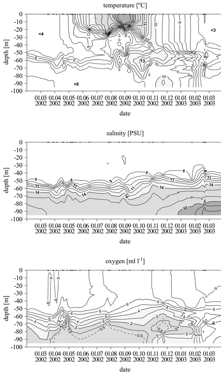
**Fig. 4.** Vertical profiles of temperature, salinity and oxygen concentration at IOW station 212 in the central Bornholm Basin, as obtained from CTD casts between February 2002 and March 2003. The two temperature maxima in early October 2002, at 60 m depth, and in mid-November 2002, at 90 m depth, mark the so-called BB60 and BB90 waters of the summer inflow
