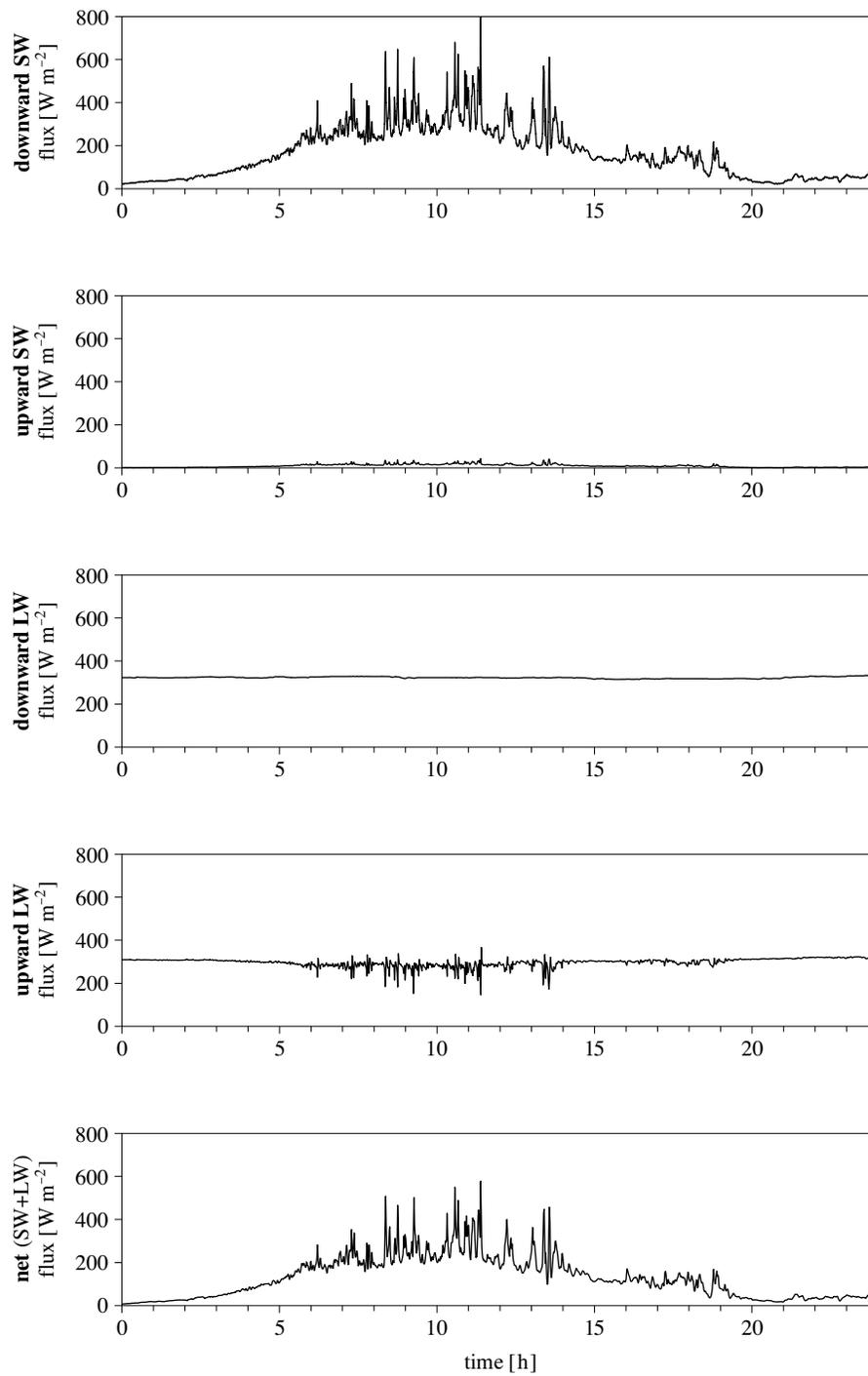
**Fig. 3.** Radiation fluxes for a selected day (04.07.2000)
