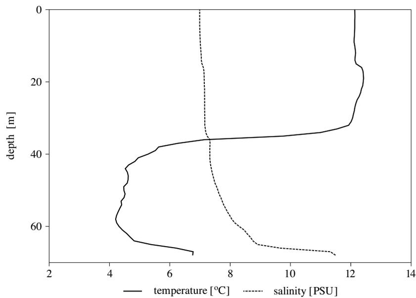
**Fig. 4.** Temperature and salinity profiles measured concurrently with echosounding
