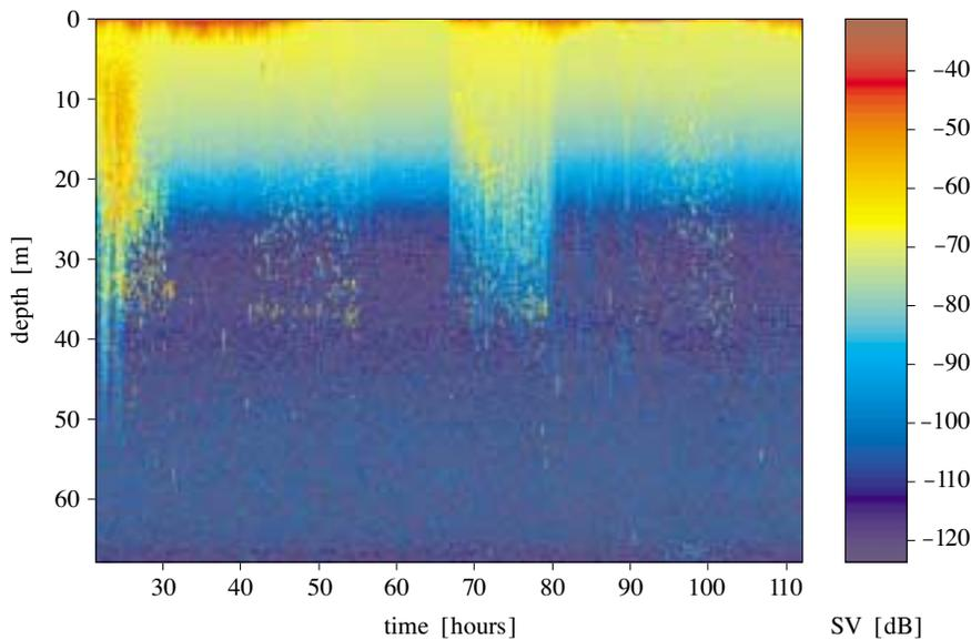
**Fig. 5.** Time-series data on volume backscattering strength collected during the 90.5 hour experiment in the Slupsk Furrow
