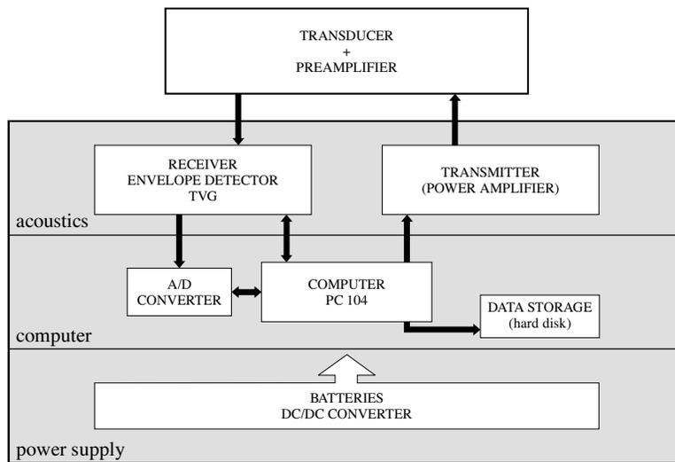
**Fig. 2.** Diagram of the electronic system
