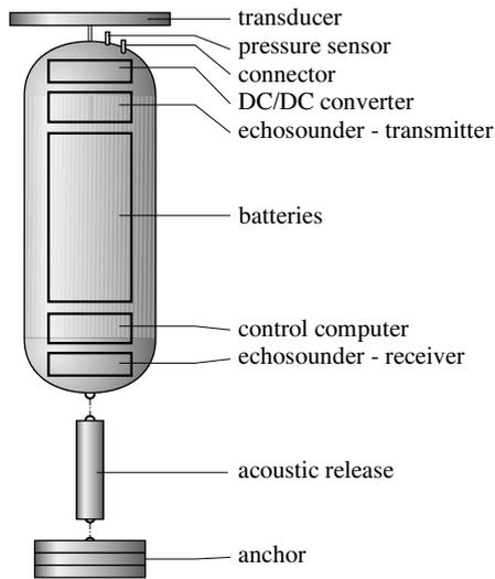
**Fig. 1.** General view of the Autonomous Hydroacoustic System
