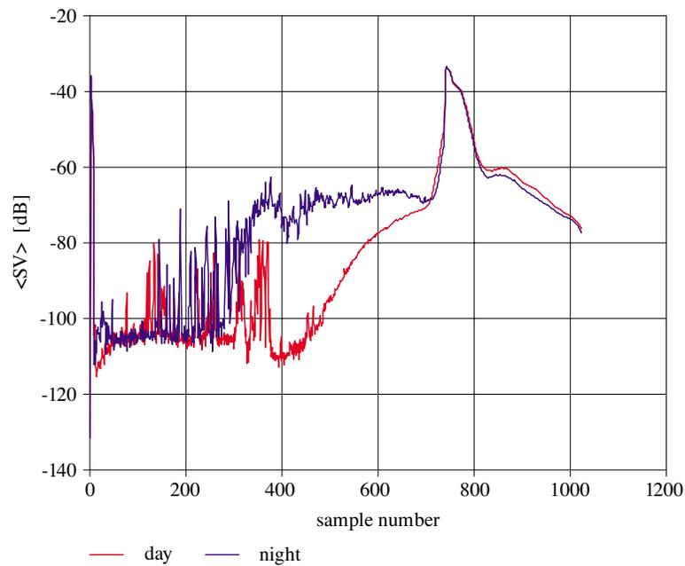
**Fig. 7.** Depth profiles of the volume backscattering strength averaged over all daily measurements (red curve) and over all night measurements (blue curve)
