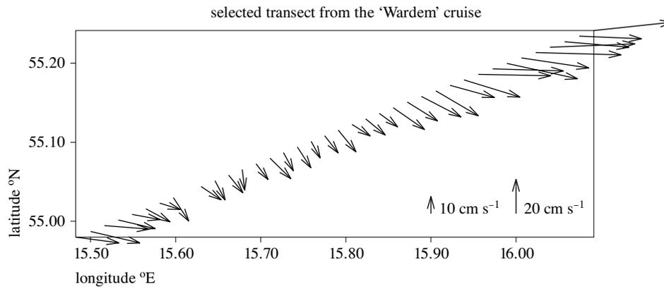
**Fig. 2.** Vectors of currents at 20 m depth with navigation as a reference
