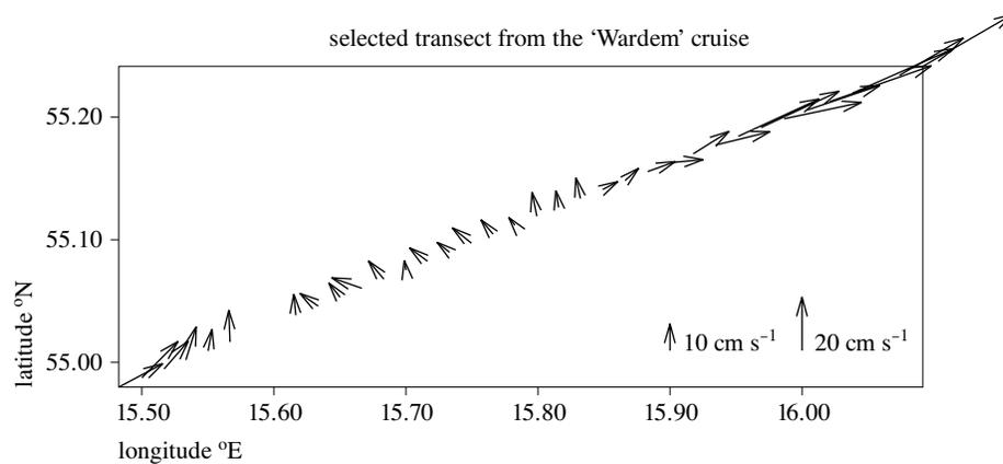
**Fig. 6.** Vectors of currents with navigation as a reference after calibration  $\alpha = -2.64$ ,  $\beta = 1.0004$
