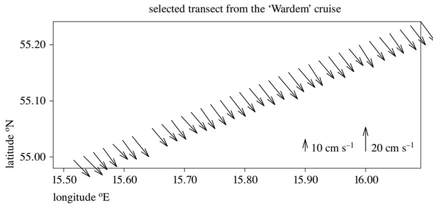
**Fig. 4.** Difference of vectors with navigation and bottom as references
