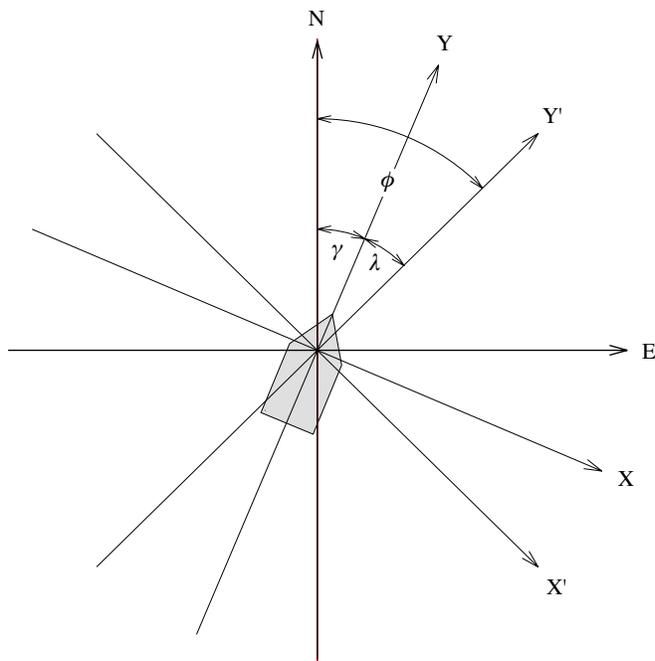
**Fig. 1.**  $OX'Y'$ : ADCP's coordinates,  $OXY$ : ship's coordinates,  $ONE$ : geographical coordinates
