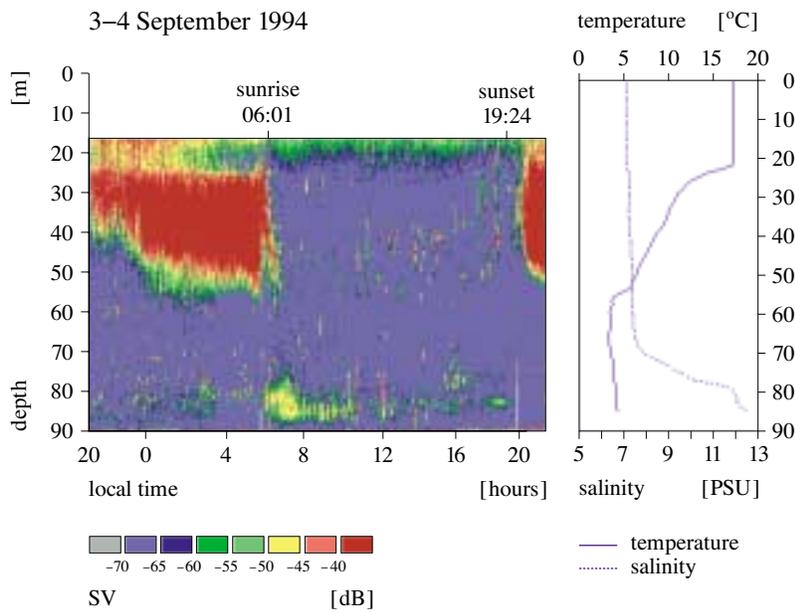
**Fig. 3.** Diurnal condensed echogram (left), temperature and salinity profiles taken at 20:00 (right) on 3 September 1994
