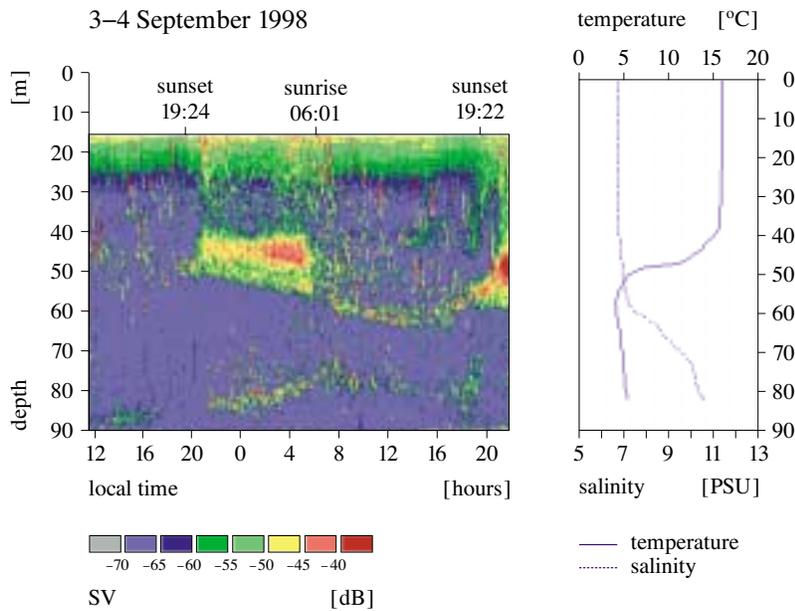
**Fig. 4.** Diurnal condensed echogram (left), temperature and salinity profiles taken at 20:00 (right) on 3 September 1998
