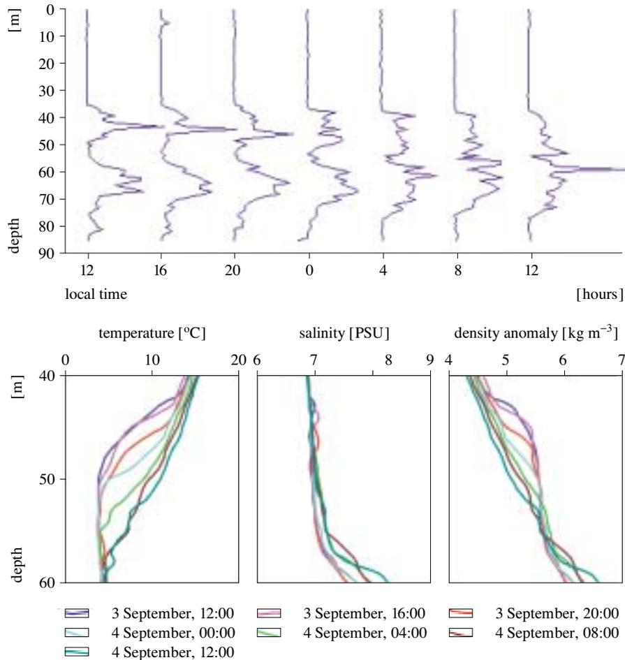
**Fig. 5.** Density gradient calculated for different instants of observation (upper), temporal changes in vertical profiles of temperature, salinity and density for the 40–60 m layer (lower) in September 1998
