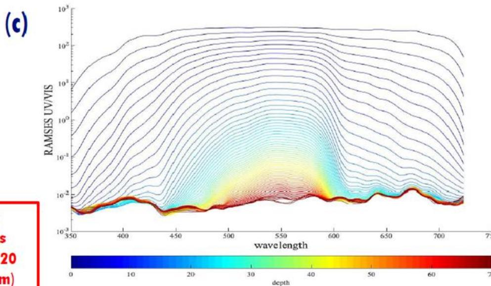
Example of RAMSES spectra (a) raw data; (b) the outliers (flagged 2 and 3) are eliminated ; (c) near surface and eliminated data are inter/extrapolated (smoothing spline/move median)
